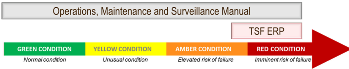
Figure 2: Conditions in a TSF operation and the relationship between ERP and OMS Manual
