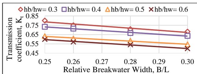
Figure 3. Effect of relative breakwater width on the reduction of wave height for different relative breakwater heights
