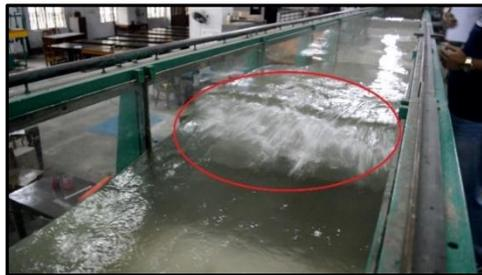
(a) Wave breaking on submerged breakwater
