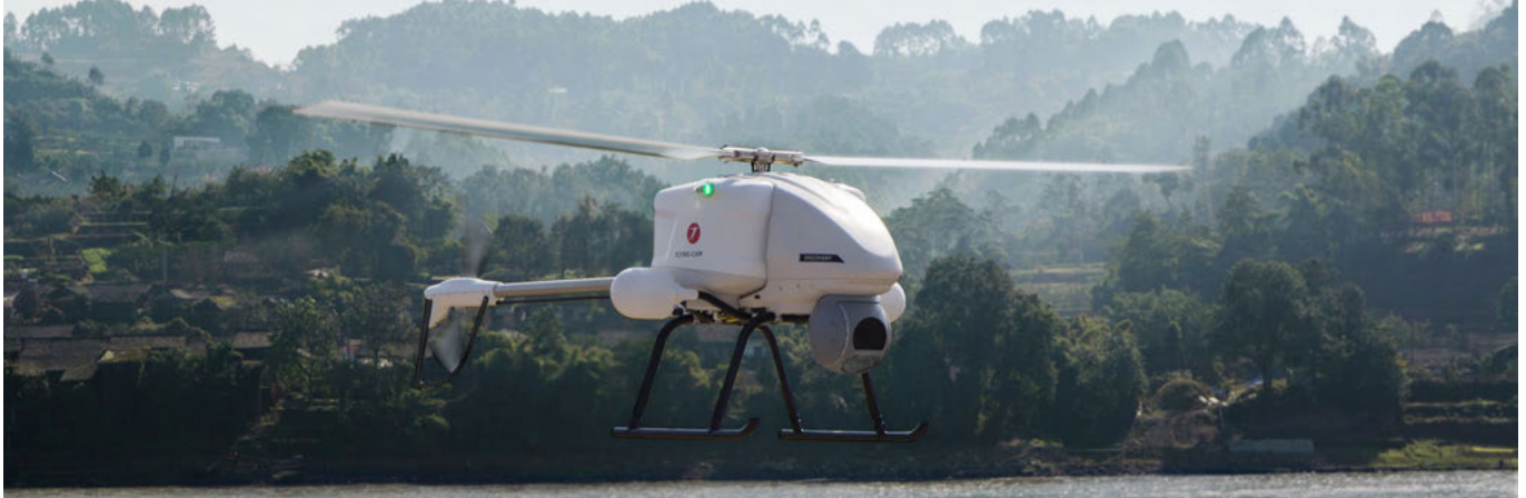
Figure 5: FLYING CAM Discovery: Advanced ultra-long-range security & surveillance unmanned aircraft system.
