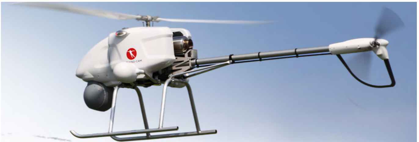
Figure 5: FLYING CAM Discovery: Advanced ultra-long-range security & surveillance unmanned aircraft system.
