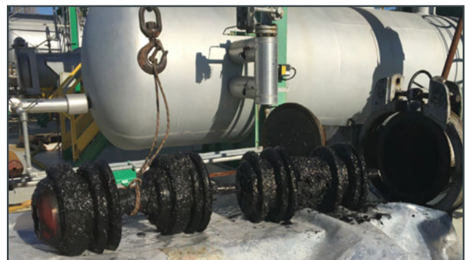
Figure 3: PIG2 Dual module heavy brush arrived at Falconara terminal.
