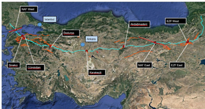
Figure 4: Fault crossings along the pipeline route; NAF – North Anatolian Fault, EZF – Erzurum Fault
