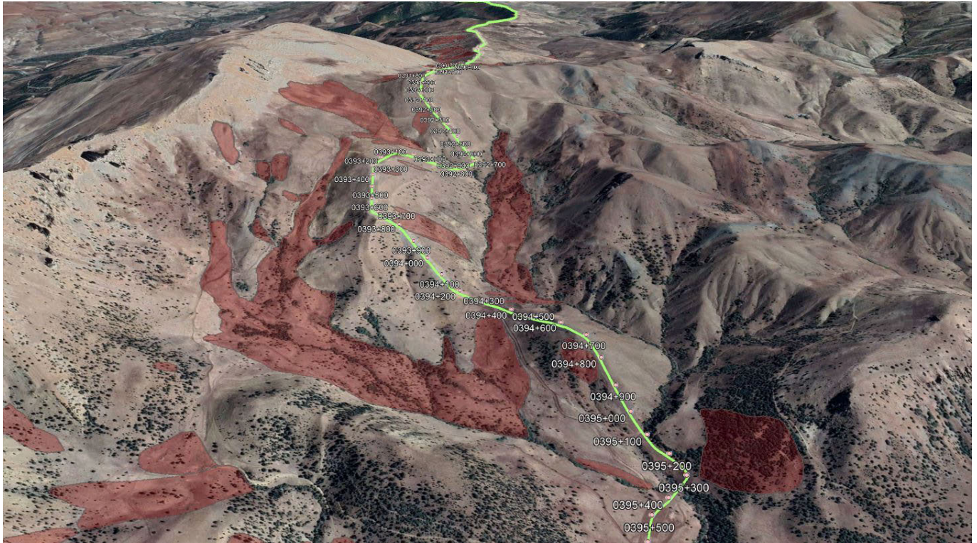
Figure 2: Landslides (areas marked in red) at Meryem Dağ mountain range, Erzincan Province, give a good example of the impact of geohazards on the alignment of TANAP.
