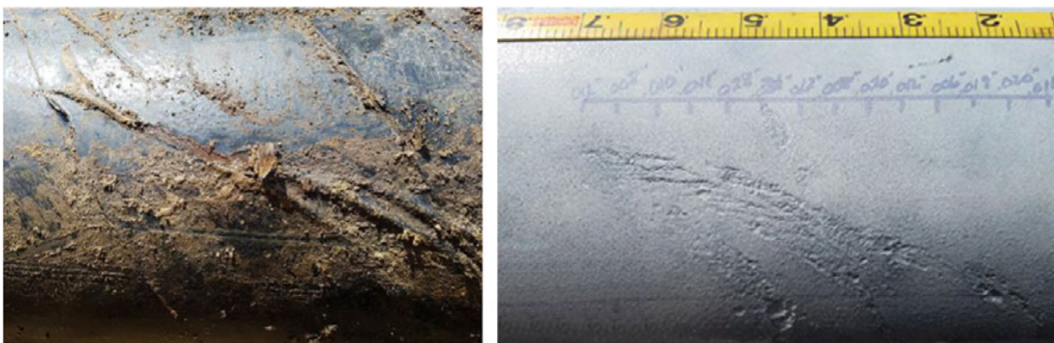
Figure 1: An example of non-axial SCC
