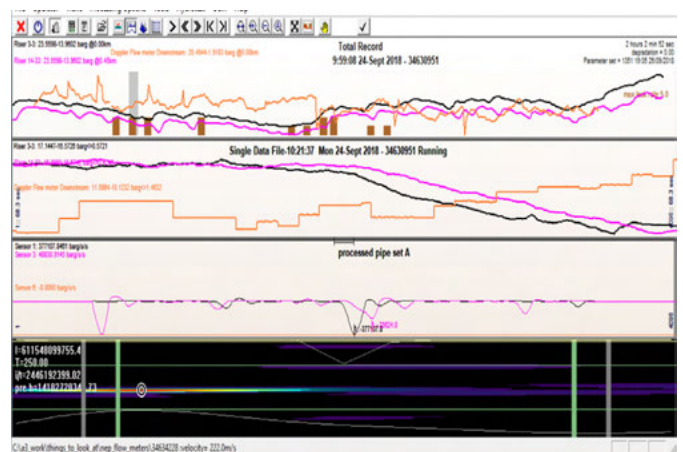
Figure 4: shows a leak detected by the Nanowave configuration
