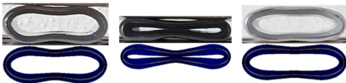
Fig. 16. The deformed shape of the PEX-Al-PEX pipe at a point during the compression, at the maximum compression, and after unloading.
