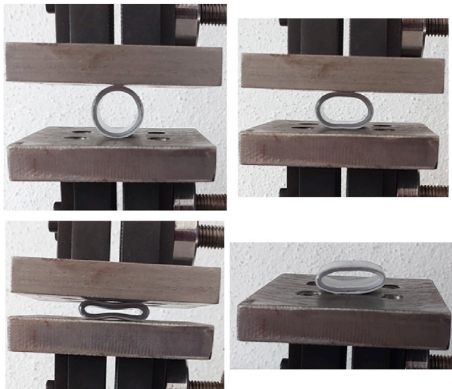
Fig. 10. Snapshots of the PEX-Al-PEX pipe compression at different time points.
