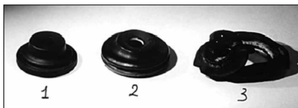
Figure 6. Example of chloramines induced elastomer degradation of a rubber components from the appliances industry.
