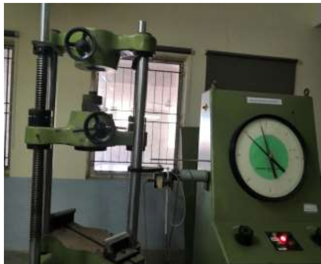
Figure 8. Universal testing machine which was used to find the compressive strength in transverse direction.
