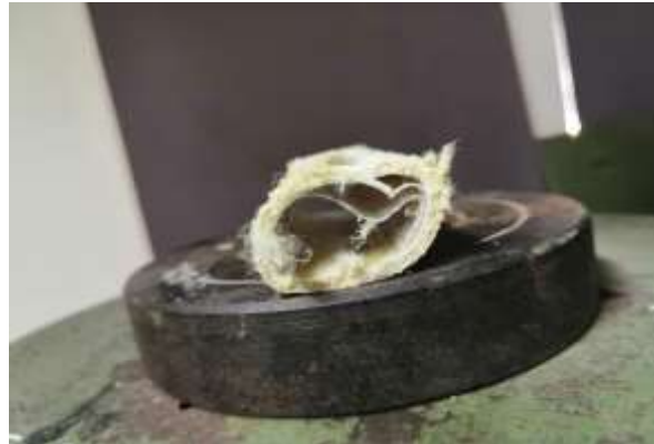
Figure 7. Tested specimen after compression test in transverse direction.
