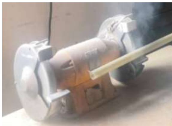
Figure 5. Grinding the edges of the fabricated kevlar composite pipe to remove irregularities.
