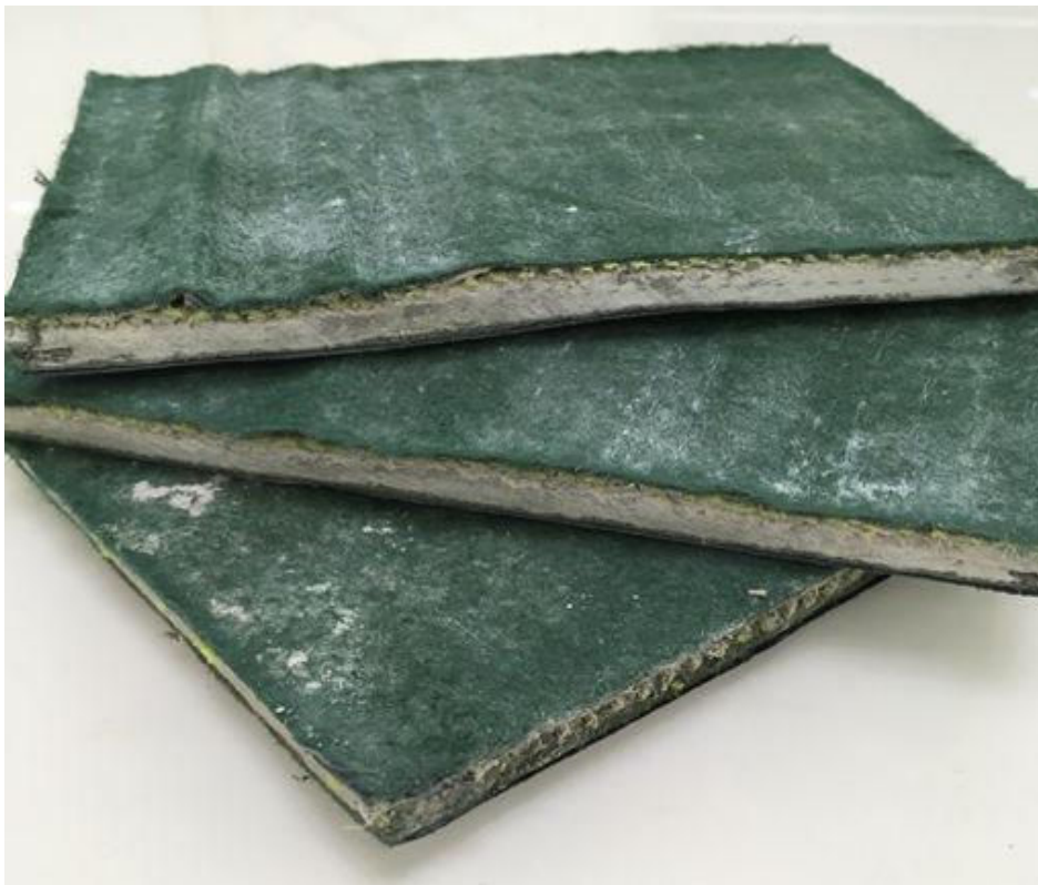
Concrete Mat Cloth GCCM CMC8 set hard sample after adding water.
