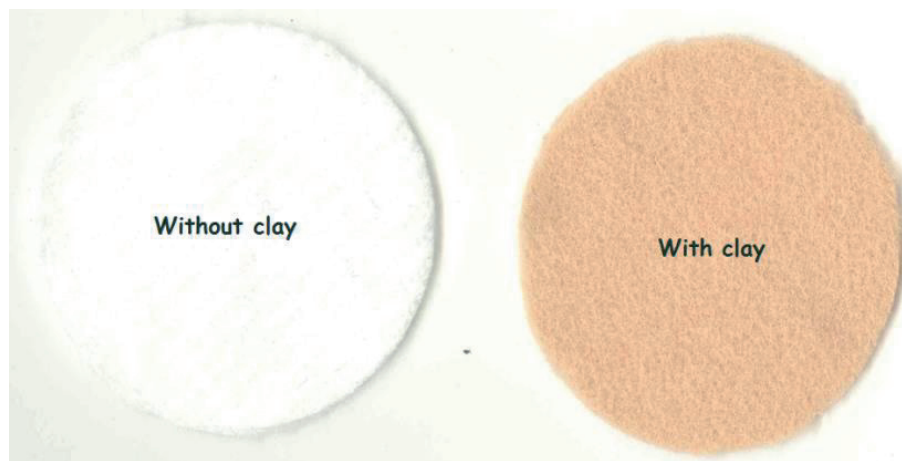
Figure 15. Clay added geotextile to improve adsorption efficiency.
