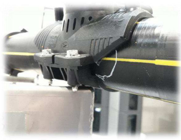
Fig. 21 Results of the hydrostatic pressure tests performed on the pipe_saddle assemblies with defects at the interface, welded at nominal time. The photo illustrates a leaking assembly resulting of a failure at the interface
