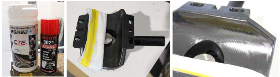
Fig. 2 Liquid contamination by applying spray on one half of the heating zone of the tapping saddle
