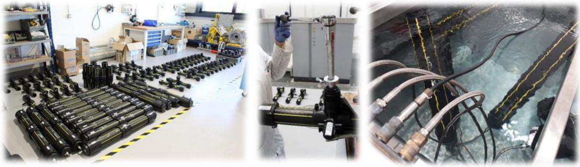
Fig. 20 Assemblies implemented for the hydrostatic pressure tests
