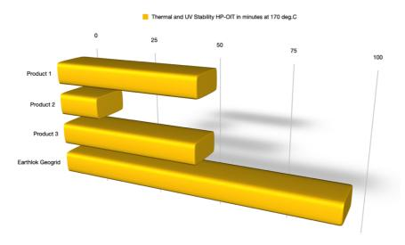
The Earthlok geogrid HP-OIT stability of 97 mins at 170 deg.C translates to 388 mins at 150 deg.C
