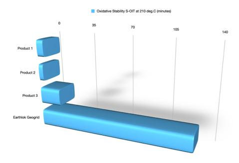
The Earthlok geogrid S-OIT stability of 128 mins at 210 deg.C translates to 256 mins at 200 deg.C
