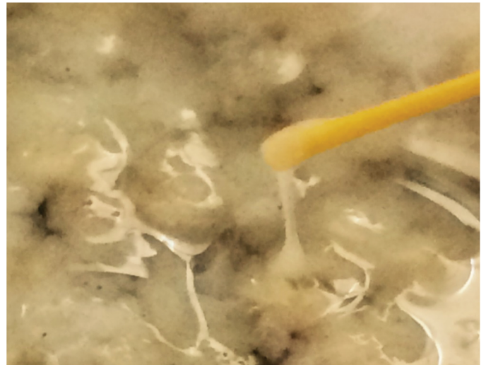
Fig. 9. (Color) Image of bentonite-polymer from CPH GCL in DI water at 20× using optical microscope; gray matter is hydrated bentonite; clear gel is polymer hydrogel
