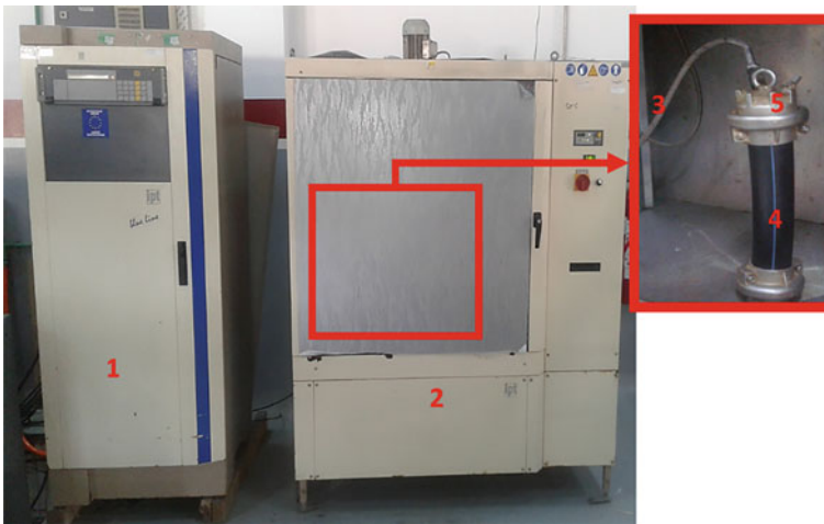
Fig. 1 The experimental platform experimental of the thermal oxidative aging test of pressured PE pipes (1-Pressure pump, 2-Oven, 3-Connection line, 4-Pipe PE100, 5-Nipple (laboratory-CTPC))
