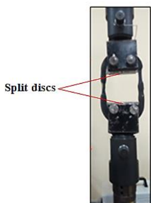
Figure 3 Nol ring test on full specimens (illustration of split discs).
