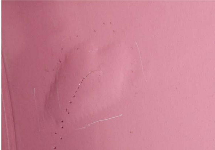
Figure 7. Typical Bulge Defect Being Drained for Repair
