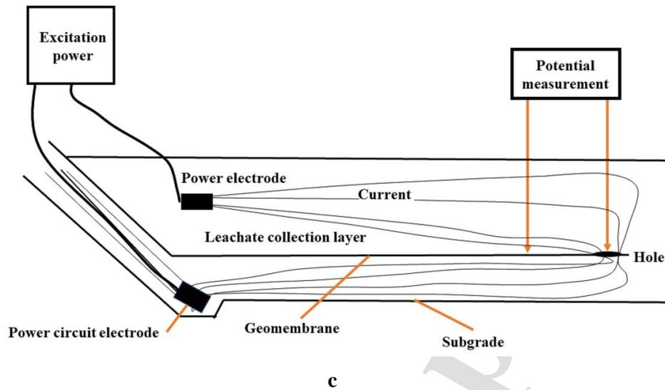
**Figure 1.** Principle diagram of (a) structure of single-layer liner system, (b) structure of double-layer liner system, (c) leakage detection by dipole method.
