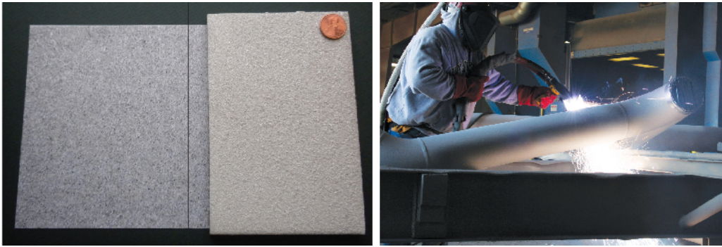
Fig. 1: Thermal spray aluminum is a single-coat instant dry CUI coating with very wide temperature tolerance and good service life. TSA requires specialized inspection after application; properly applied TSA is nearly identical in appearance to fresh white-metal blasted steel. The sample panel with the penny is the TSA. Photos: Courtesy of the Author
