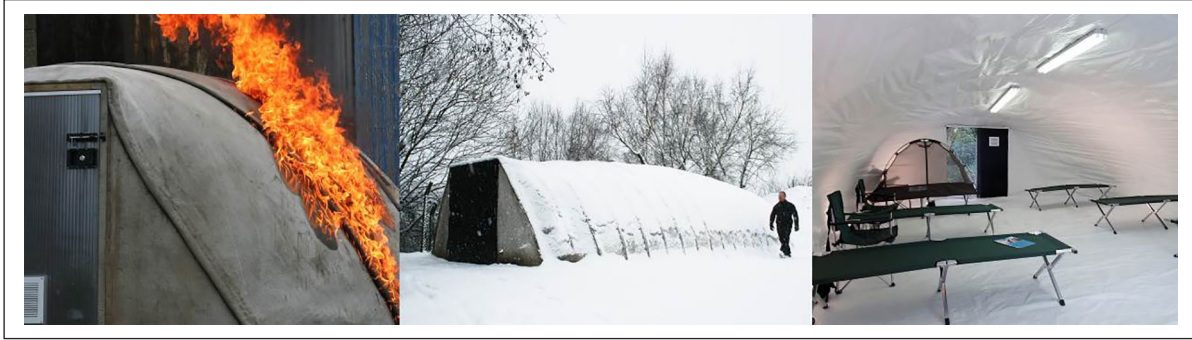
Figure 4. Protective performance test and interior view of concrete canvas tent.
