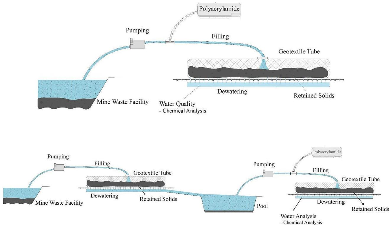
**Fig. 12** Dewatering alternative with **a** single geotextile tube and **b** two geotextile tubes
