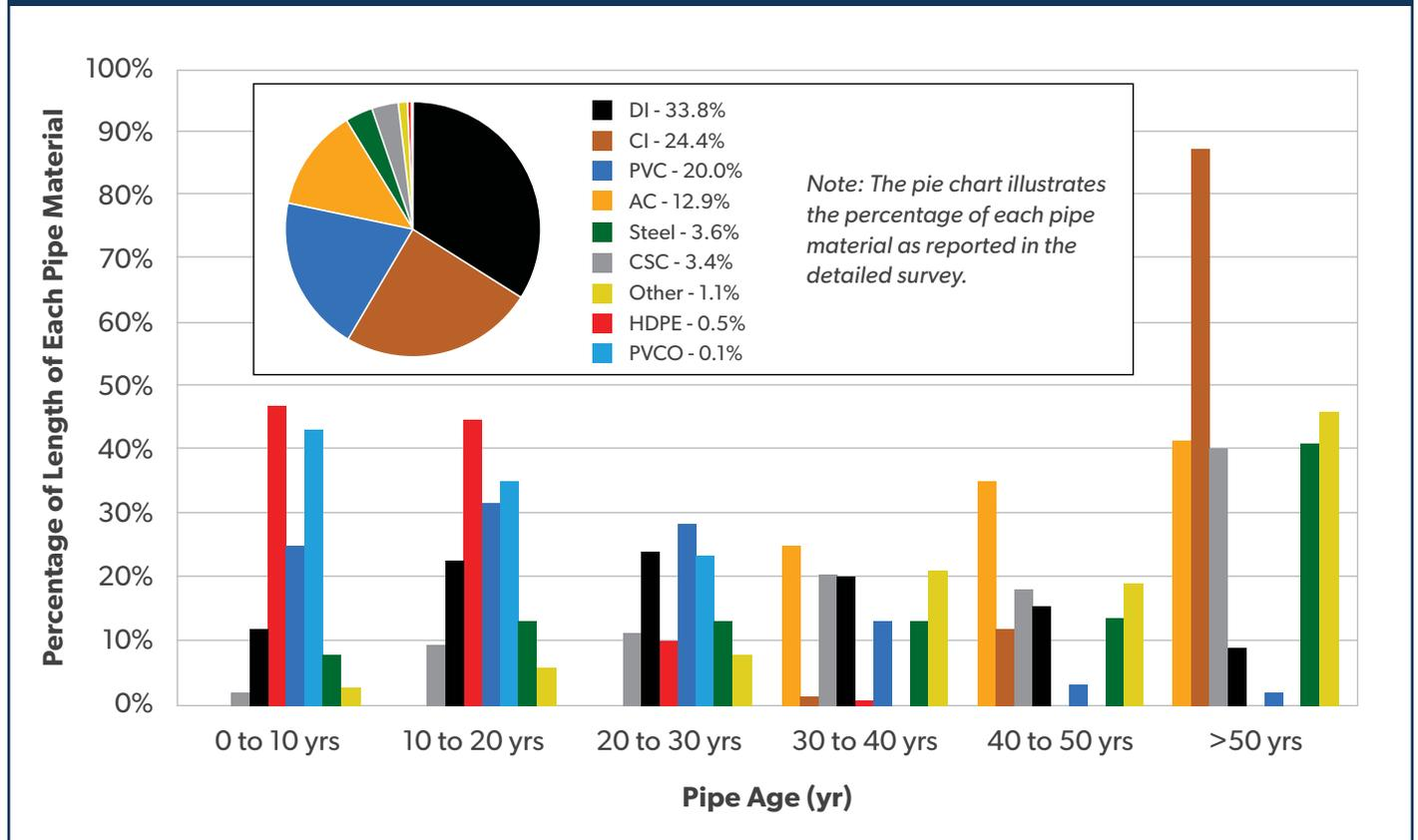
Figure 22 shows the age distribution as a percentage of the total length of all pipe materials from the detailed survey. For example, CI older than 50 years is 21% of all installed pipe. For ages between 0 to 10 years, DI and PVC both have about 4 to 5% of the total installed length. This means that the most common pipe materials installed over the last 10 years are DI and PVC.
