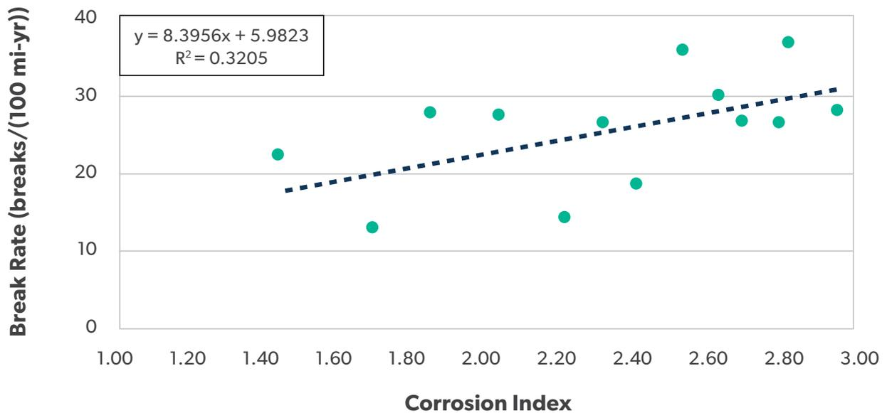
FIGURE 46: DUCTILE IRON PIPE BREAK RATE BY CORROSION INDEX (BASIC SURVEY)
