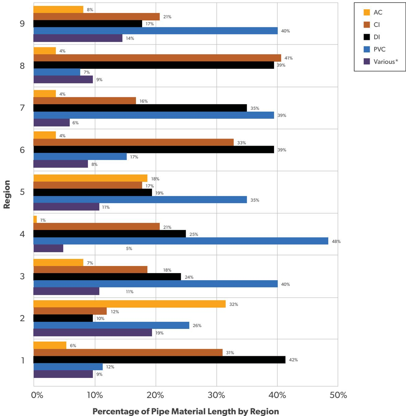
\*The "Various" category combines all pipe materials that are at 3% and below of the total pipe length, which includes: CSC (2.8%), HDPE (0.6%), PVC0 (0.1%), Steel (2.8%), Other (1.1%), and Unknown (3.0%).
