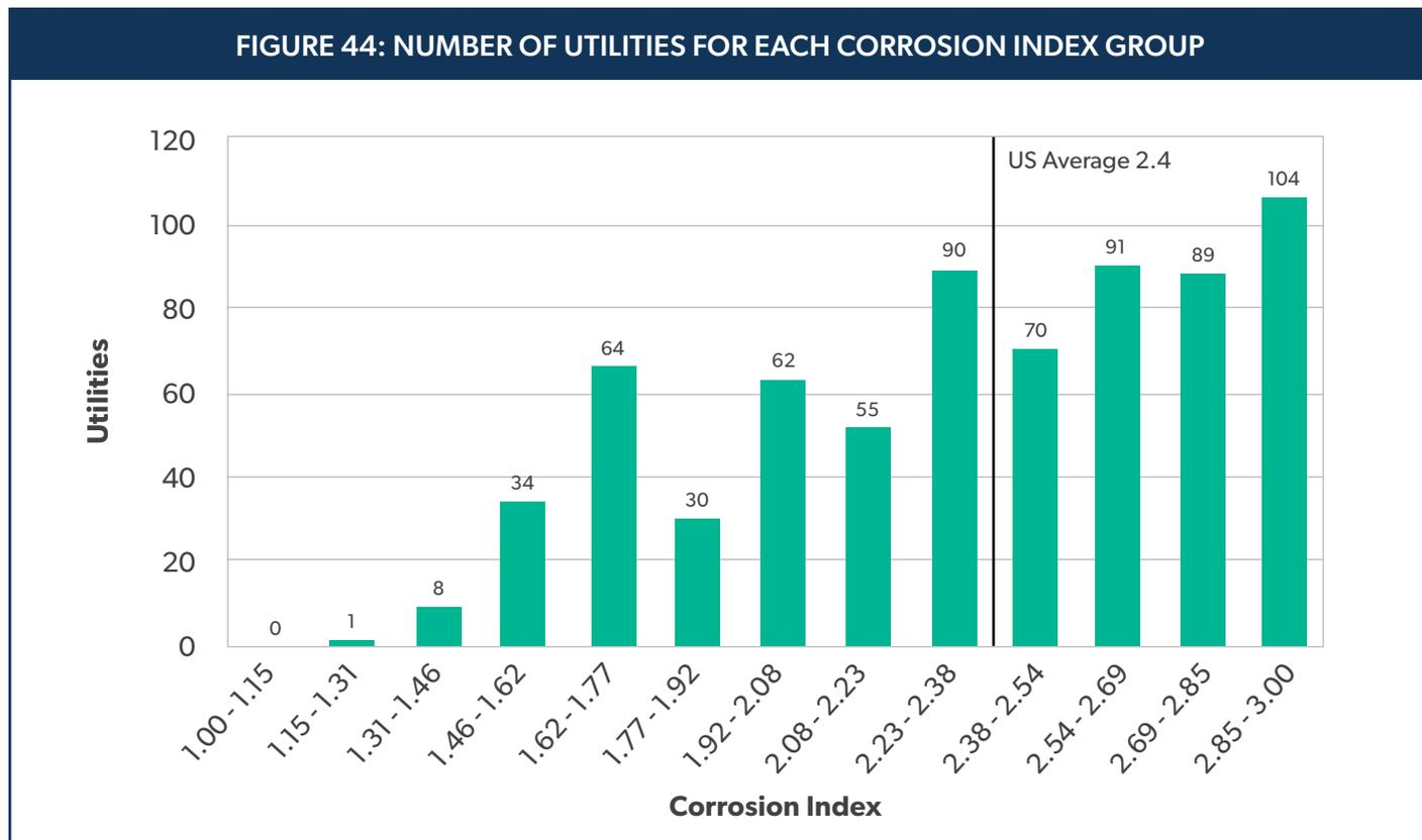
The average corrosion index for all the US utilities in the basic survey was found to be 2.37 or close to midway between moderate and high corrosion risk. Notably, the overall corrosion index of the US from Figure 44 is 2.4. That is, most utilities in the US have a moderate to high soil corrosion risk, which is consistent with the detailed survey report that showed 75% of utilities have one or more areas with corrosive soil.
