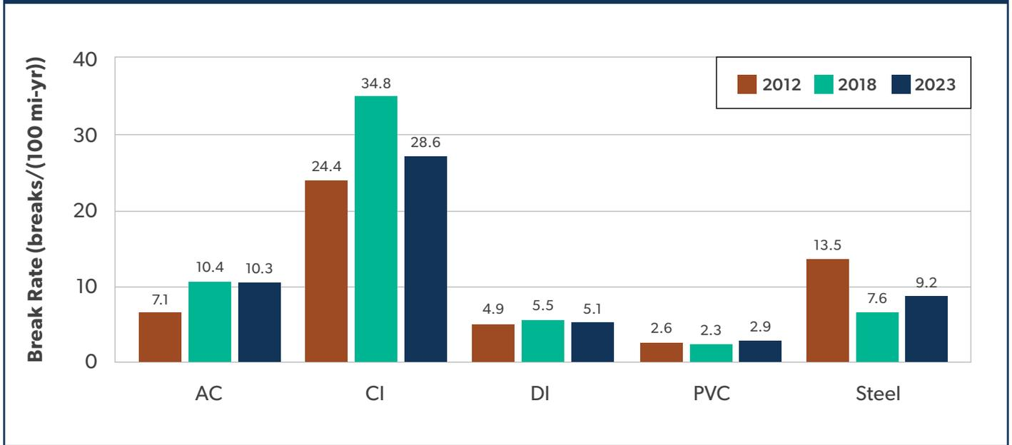
**FIGURE 32: COMPARISON OF BREAK RATES FROM THE 2018 AND 2023 BASIC SURVEYS FROM THE SAME 151 UTILITIES**
