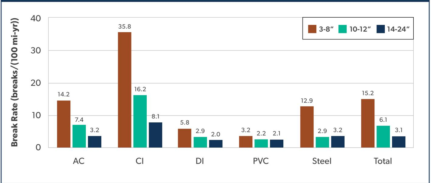
Figure 39 illustrates the break rate of 3- to 12-inch pipe, while Figure 40 indicates the break rates of 3- to 8-inch pipe. Comparing these two figures shows a small difference in break rates. The 3- to 12-inch diameter range represents 86% of all pipe materials.
