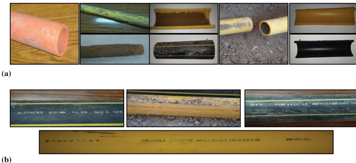
Fig. 1 Samples of extracted polyethylene pipes. (a) Polyethylene pipes before cleaning. (b) Polyethylene pipes marking. (The color of the printed information is different from the basic color of the pipes.)
