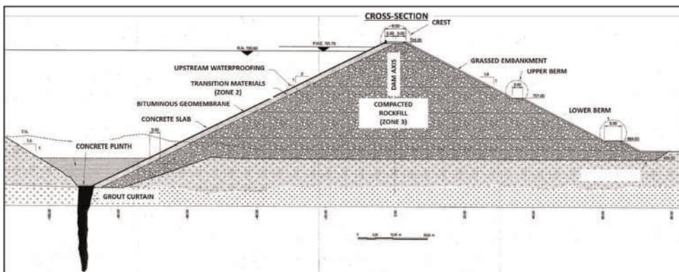
Figure 1. Typical cross-section of La Galaube dam (ISL).
