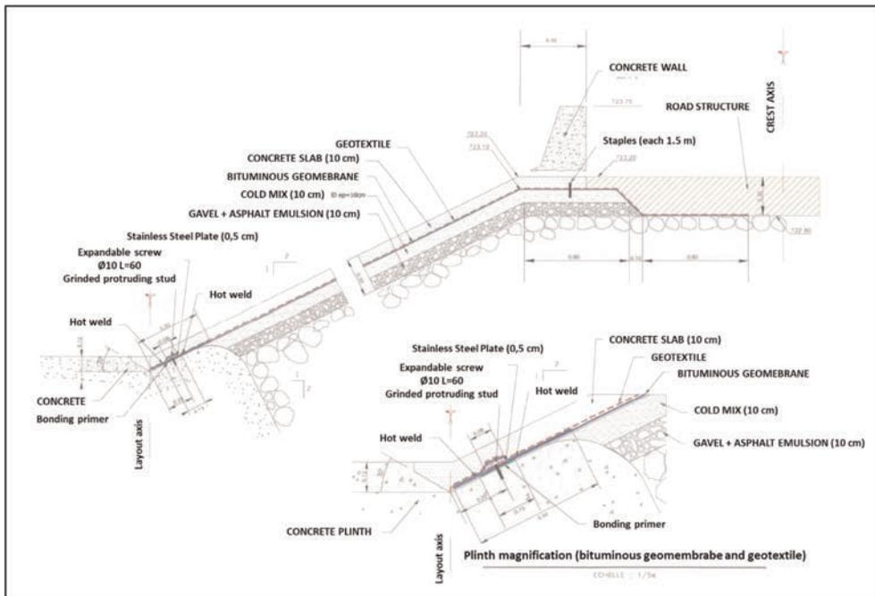
Figure 2. Typical cross-section of the upstream facing.
