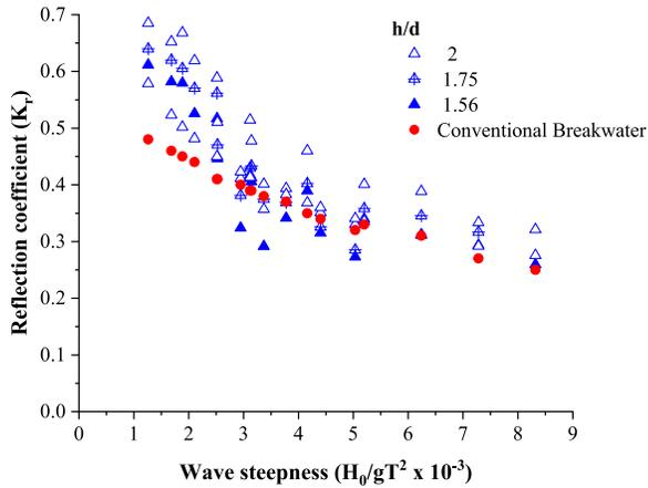
**Fig. 10.** Reflection coefficient ( $K_r$ ) values with respect to wave steepness for all the test cases conducted for Bag 1.
