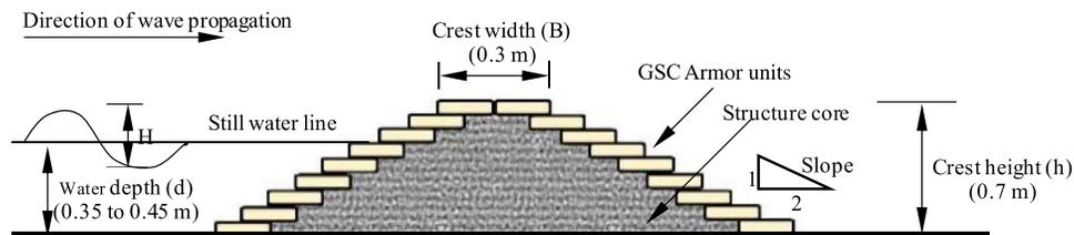
Fig. 1. Schematic diagram of GSC breakwater model.
