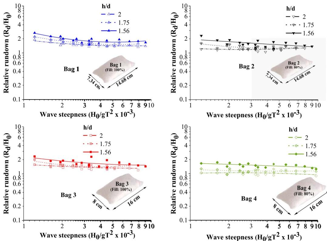
Fig. 7. Variation of relative rundown of various configurations for different relative water depths.
