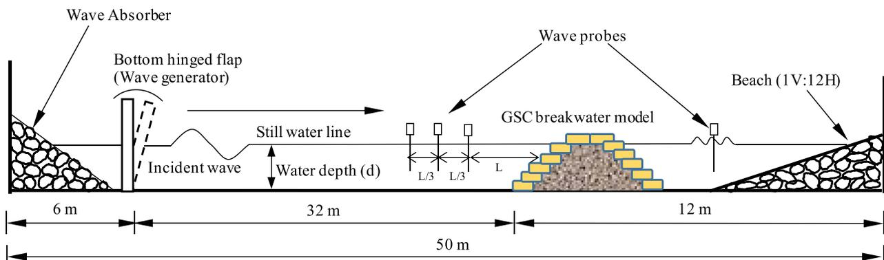
**Fig. 3.** Schematic representation of GSC breakwater model at Wave Mechanics Laboratory, NITK.
