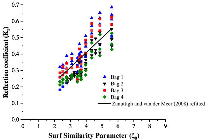
**Fig. 15.** Comparison of refitted Eq. (3) with entire range of experimental data.
