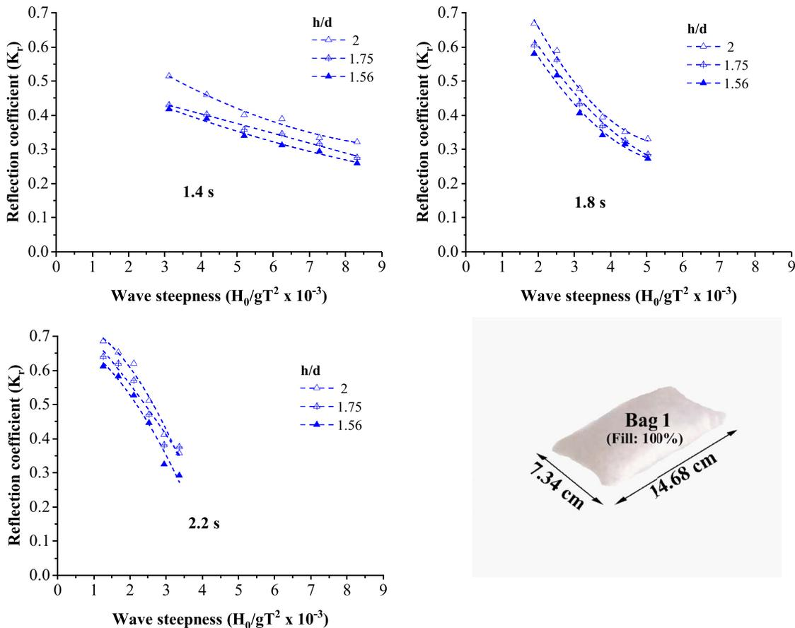
**Fig. 11.** Plots showing dependence of wave period on reflection coefficient for different configurations of GSC breakwaters stacked with Bag 1.
