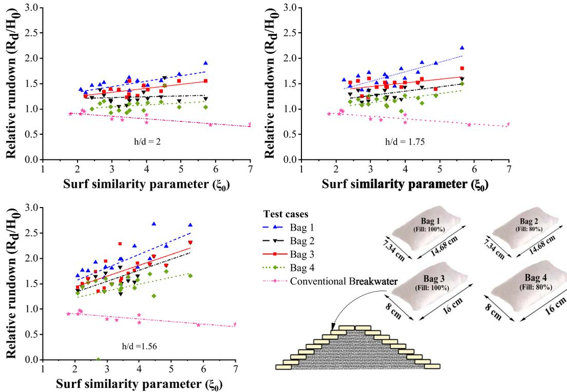
Fig. 9. Variation of relative rundown of different configurations with surf similarity parameter.
