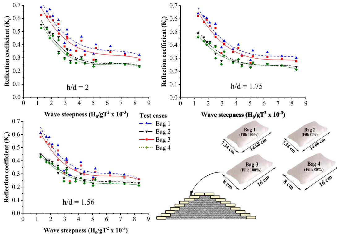
**Fig. 16.** Reflection curves of different configurations of GSC breakwaters for varying relative water depths.
