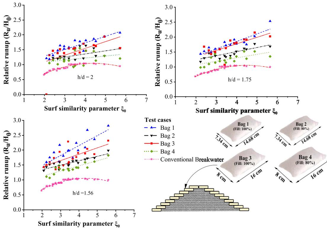
Fig. 8. Variation of relative runup of different configurations with surf similarity parameter.
