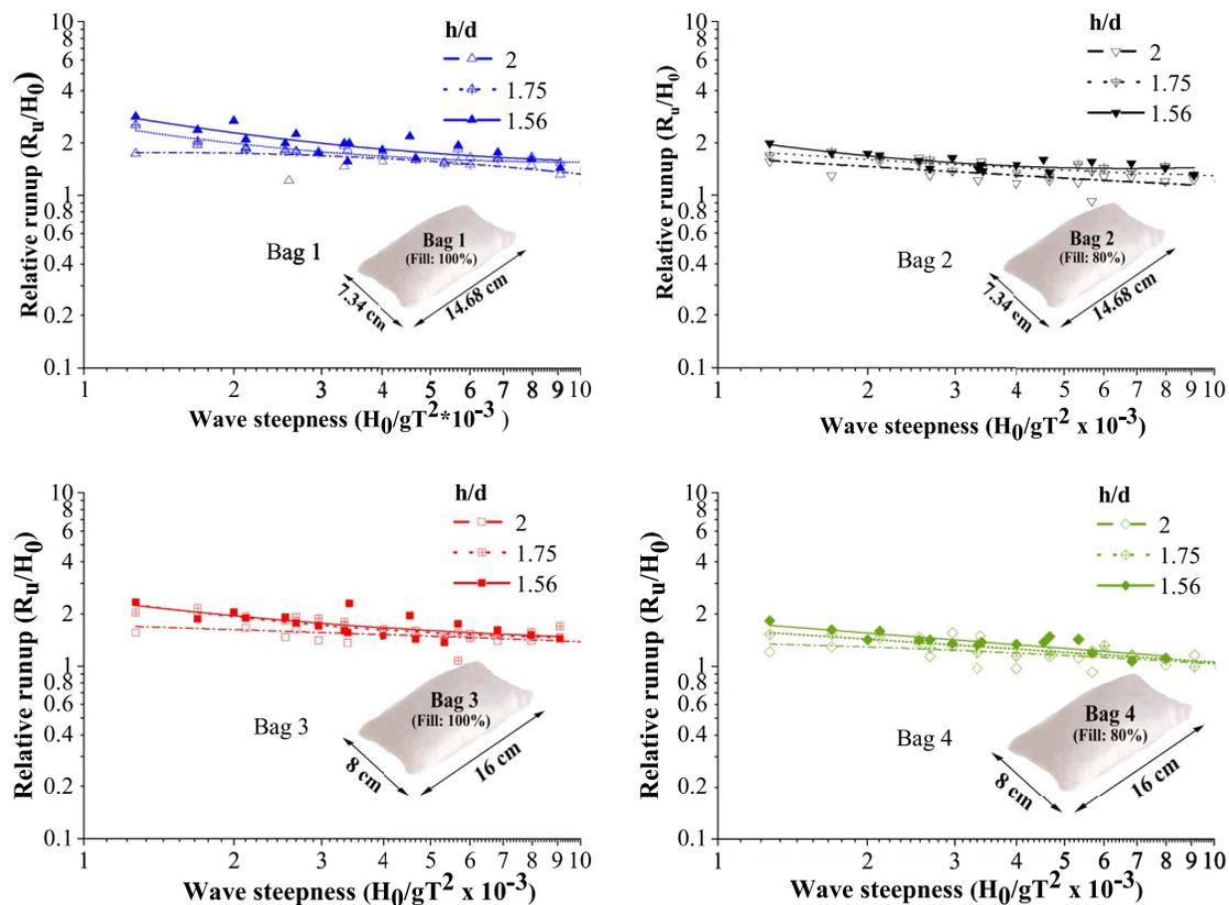
**Fig. 6.** Variation of relative runup of various configurations for different relative water depths.
