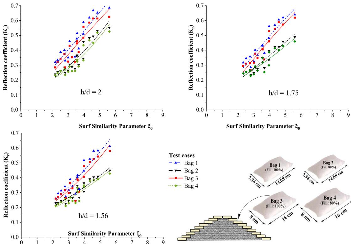
**Fig. 13.** Variation of reflection coefficient with respect to surf similarity parameter.
