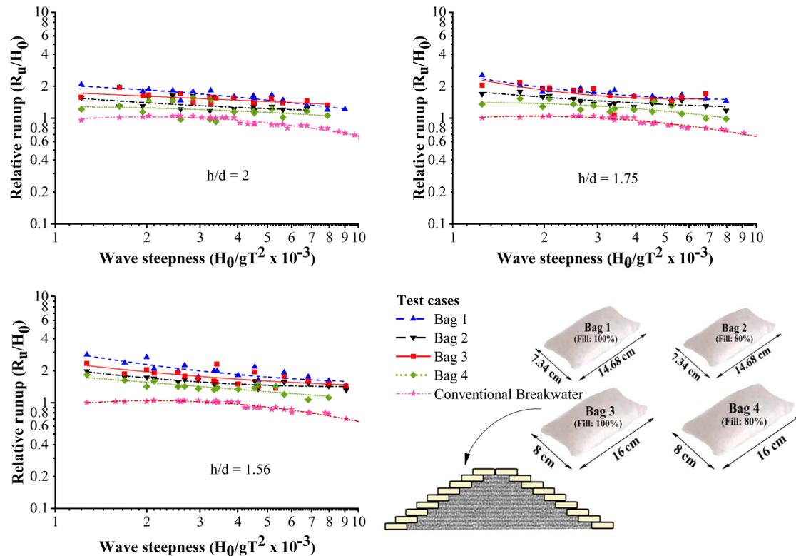
**Fig. 4.** Variation of relative runup ( $R_r/H_0$ ) with respect to deep water wave steepness ( $H_0/gT^2$ ) for various relative water depths ( $h/d$ ) for different configurations of geotextile breakwater.
