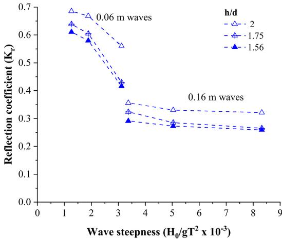
**Fig. 12.** Variation of reflection coefficient of Bag 1 with respect to wave steepness (incident wave height 0.06 and 0.16 m) for different relative water depths.
