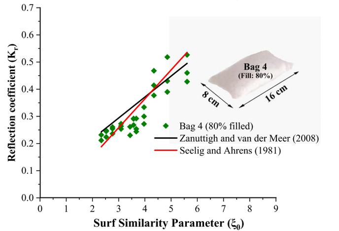
**Fig. 14.** Comparison of the experimental results with the existing reflection coefficient formulas proposed by Seelig and Ahrens (1981) and Zanuttigh and van der Meer (2008).
