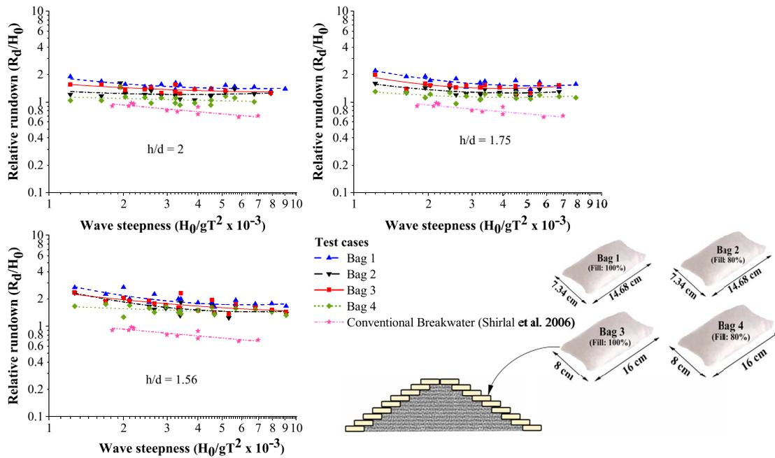
**Fig. 5.** Variation of relative rundown ( $R_d/H_0$ ) with respect to deepwater wave steepness ( $H_0/gT^2$ ) for various relative water depths ( $d/gT^2$ ) for different configurations of geotextile breakwater.
