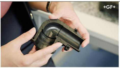
The importance of training - a failed electrofusion welding (90% of all claims are due to failed jointing technology).
