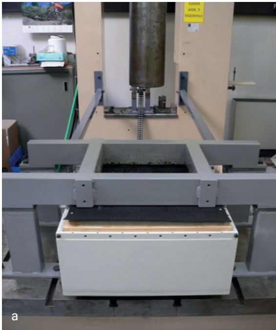
FIGURE 1: Test apparatus: (a) Direct Shear Test; (b) Inclined Plane.
