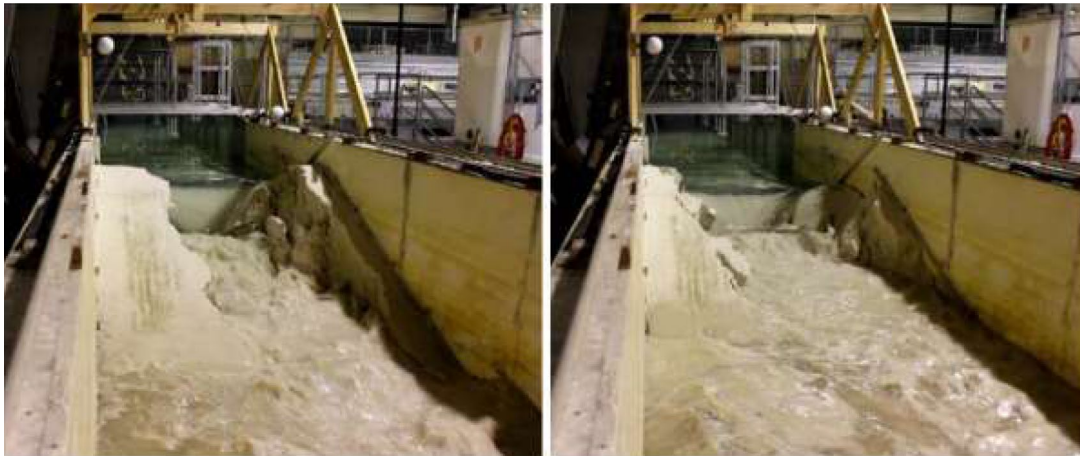
Fig. 12 Downstream oblique view of a typical dam during breach (Source: Walsh et al. 2019)
