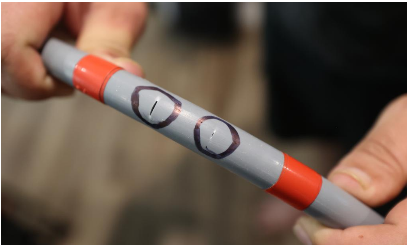
📷 Thousands of WA homeowners impacted by the defective Iplex pipe saga. Pictured - Split pipe from the damaged bathroom Credit: Daniel Wilkins/The West Australian
