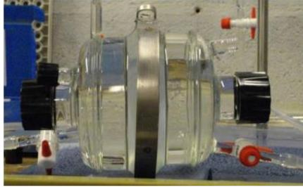
Figure 1: dual cell permeameter (overview)
