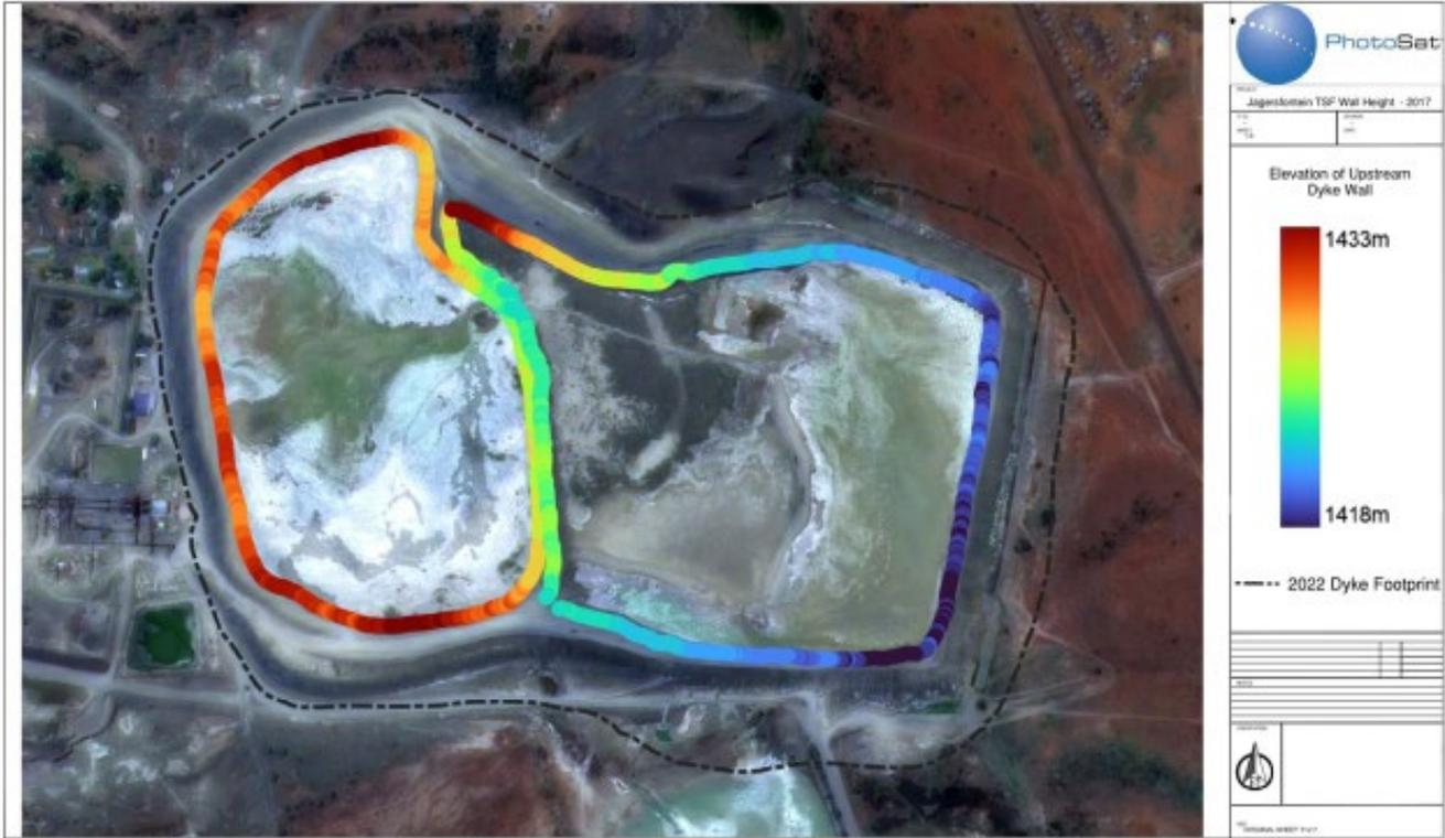
Figure 43: TSF upstream wall height for 2017
