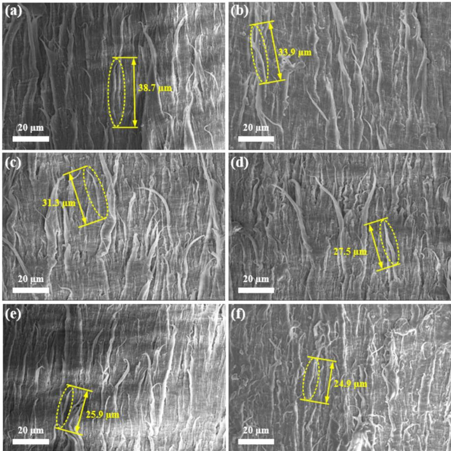
**Fig. 7** Micro-surface morphologies of fractured surfaces of butt-fusion welded joints at different aging times of thermal-oxidative aging at 90 °C. (a) 0 h, (b) 120 h, (c) 240 h, (d) 360 h, (e) 480 h, and (f) 600 h (Color figure online)
