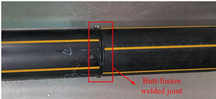
**Fig. 1** Experimental PE100 pipe with a butt-fusion welded joint (Color figure online)
