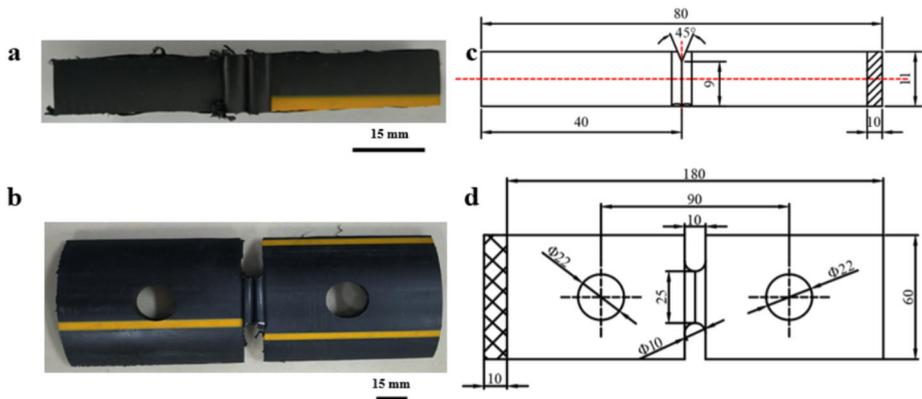
**Fig. 3** Test specimens. (a) Photograph of a sample for impact test. (b) Photograph of a sample for tensile strength. (c) Scheme of the sample size for impact test. (d) Scheme of the sample size for tensile strength (Color figure online)
