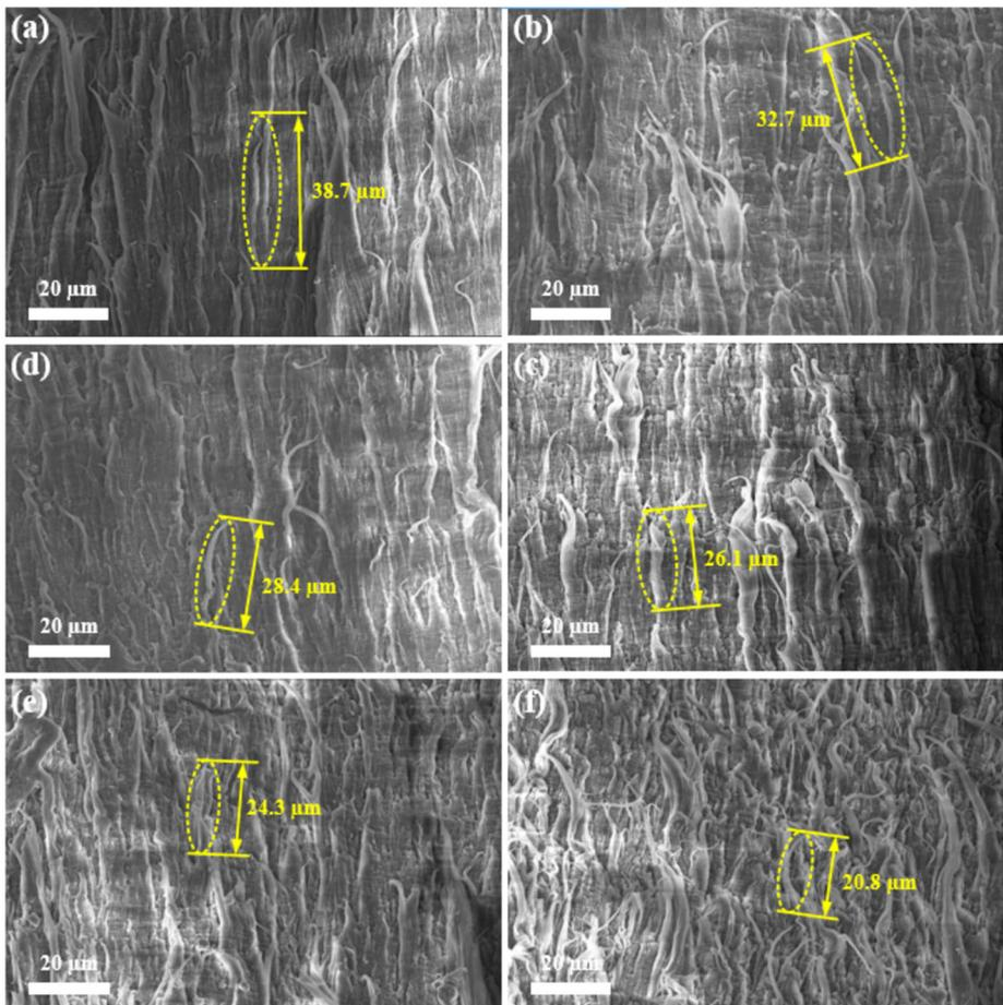
**Fig. 8** Micro-surface morphologies of fractured surfaces of butt-fusion welded joints at different aging times of thermal-oxidative aging at 120 °C. (a) 0 h, (b) 120 h, (c) 240 h, (d) 360 h, (e) 480 h, and (f) 600 h (Color figure online)
