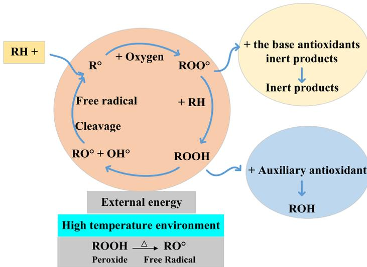
Fig. 9 Oxidative pyrolysis mechanism of high-density polyethylene (Color figure online)
