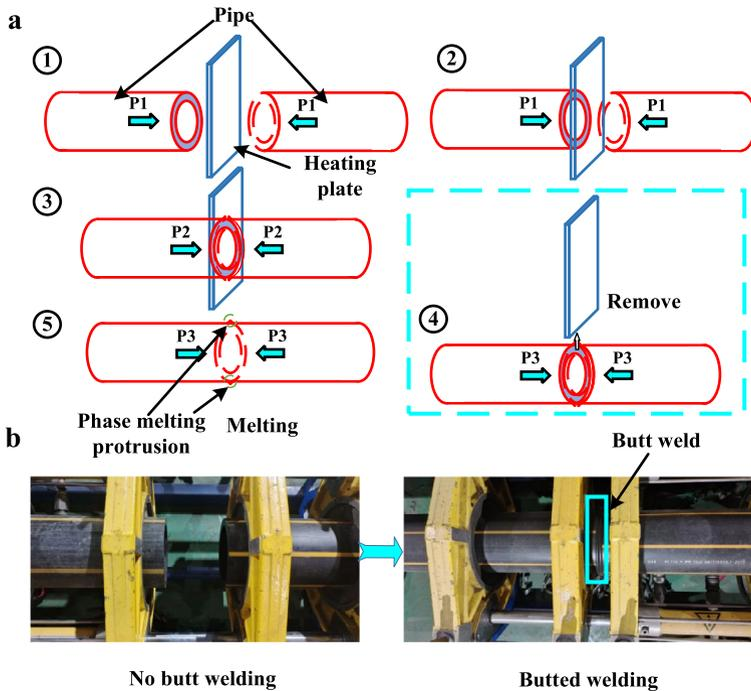
**Fig. 2** Schematic diagram of HDPE pipe butt-fusion welded joint manufacturing process and molecular chain reaction mechanism during HDPE butt-fusion welded joint production. (a) Schematic diagram of pipeline butt-fusion welded joint manufacturing process. (b) Photos of pipe butt-fusion welded joint production process (Color figure online)
