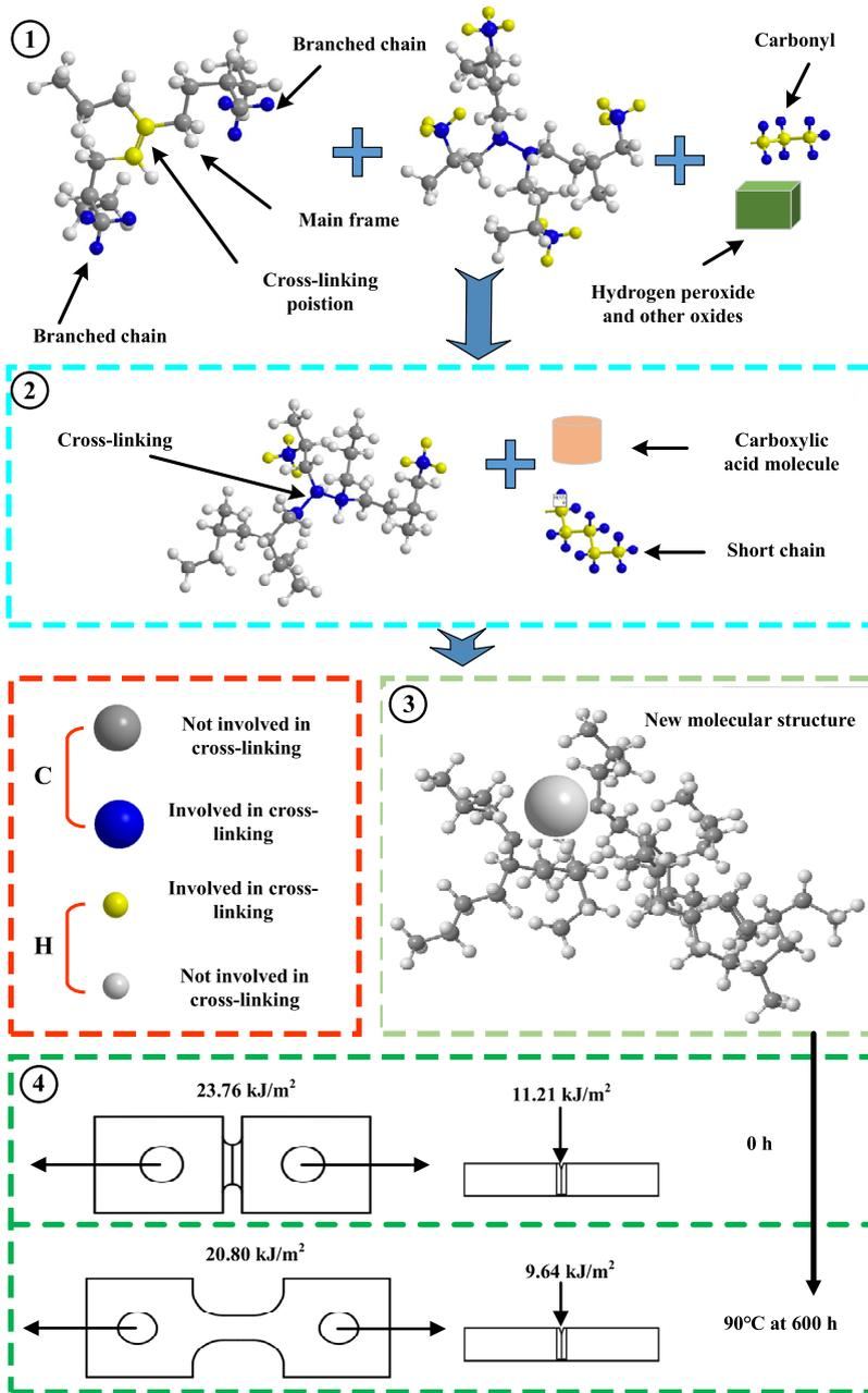
Fig. 12 Molecular chain reaction mechanism of thermal-oxidative aging (Color figure online)
