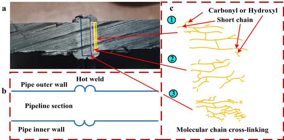
**Fig. 11** Schematic diagram of the degree of cross-linking of different areas at the melting point of HDPE pipe butt-fusion welded joint. (a) Sectional photo of HDPE pipe with butt-fusion welded joint. (b) Section diagram of HDPE pipe with butt-fusion welded joint. (c) Schematic diagram of the degree of cross-linking of different areas at the melting point of HDPE pipe with butt-fusion welded joint (Color figure online)
