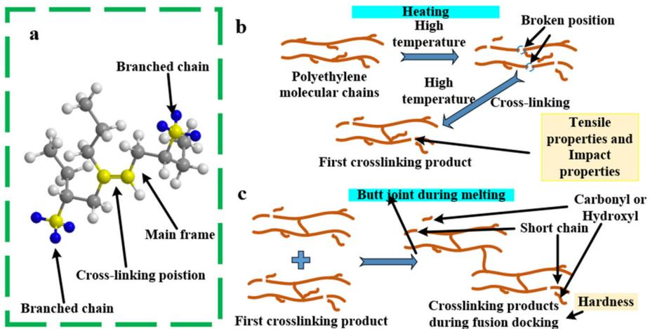
Fig. 10 Molecular chain reaction mechanism during HDPE butt-fusion welded joint production. (a) Molecular diagram of HDPE butt-fusion welded joint. (b) Schematic diagram of molecular chain change after heating of HDPE butt-fusion welded joint. (c) Schematic diagram of change in the molecular chain after HDPE butt-fusion welded joint (Color figure online)
