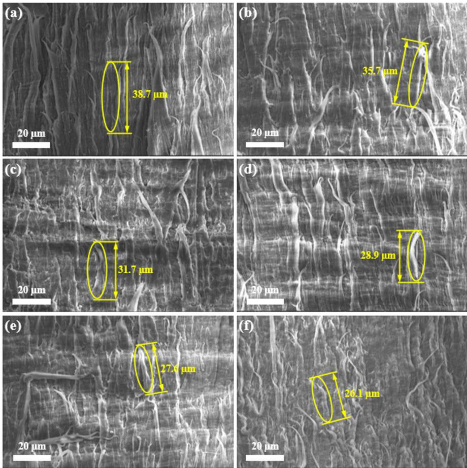
**Fig. 6** Micro-surface morphologies of fractured surfaces of butt-fusion welded joints at different aging times of thermal-oxidative aging at 60 °C. (a) 0 h, (b) 120 h, (c) 240 h, (d) 360 h, (e) 480 h, and (f) 600 h (Color figure online)
