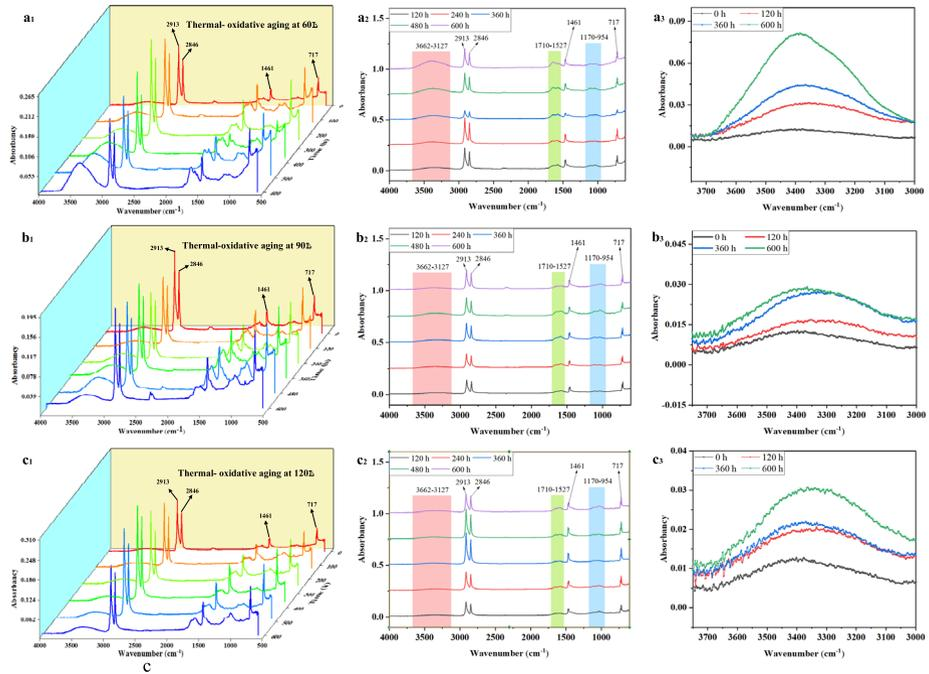
**Fig. 5** FTIR absorbance spectra of butt-fusion welded joint after thermal-oxidative aging at different times. (a<sub>j</sub>) Thermal oxidative aging at 60 °C. (b<sub>j</sub>) Thermal oxidative aging at 90 °C. (c<sub>j</sub>) Thermal oxidative aging at 120 °C (j=1, 2, 3) (Color figure online)
