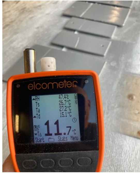
Application atmospherics were RH = 47%. Surface temperature of 26.7°C (11.7°C above dew point)
