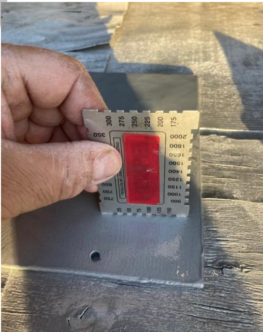
Application atmospherics were RH = 47%. Surface temperature of 26.7°C (11.7°C above dew point)
