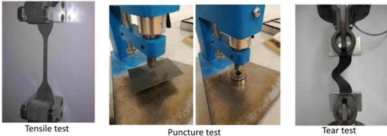
Figure 2 Picture of the mechanical tests performed on the membranes and HDPE products
