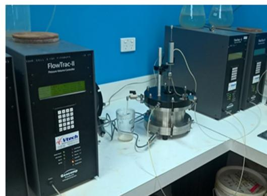
Figure 1 (a) Laboratory setup of the Rowe cell; (b) The cell used in the experiments
