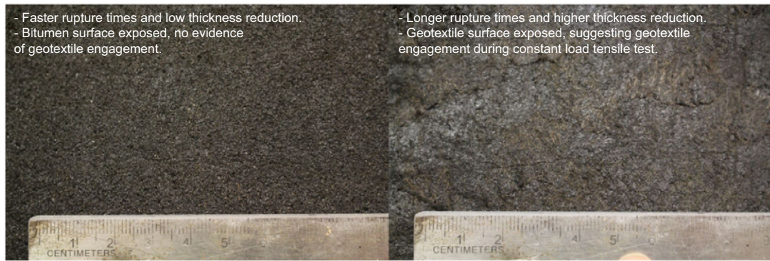
Figure 4. Constant tensile load failure surfaces of the 0.1 mm and 0.4 mm thickness reduction BGM seams. In the 0.4 mm thickness reduction case, a rough exposed geotextile surface was present after testing, with fibers oriented in the direction of applied load. This was absent in the 0.1 mm thickness reduction seam. Given the order of magnitude difference in failure time between these seams, these failure surfaces suggest geotextile engagement played an important roll in seam failure time
