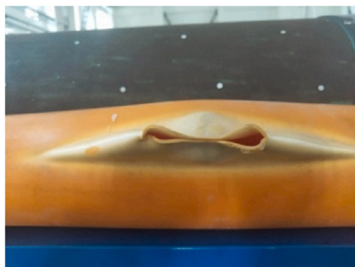
Fig. 3. The ductile failure of PE pipe subjected to internal pressure.
