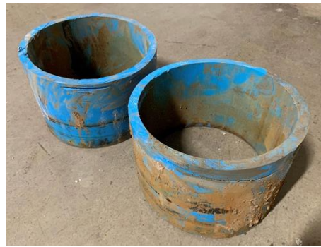
Figure 5. Excavated Samples of 8” AWWA C900 Water Main for Dimension Measurement
