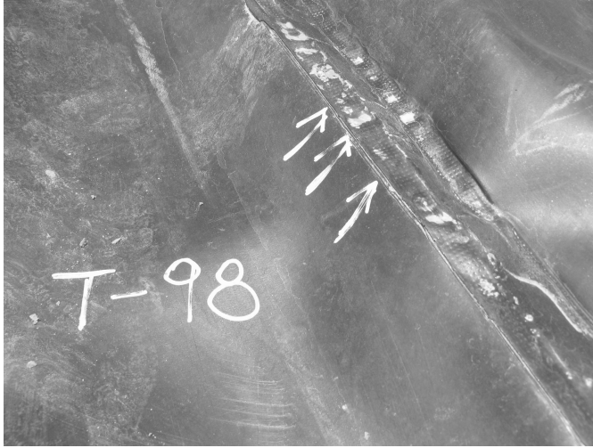
Figure 17.18 Photograph of a heat-affected weld in a 1 mm HDPE liner (note the buckling and distortion at the right side of the photograph)
