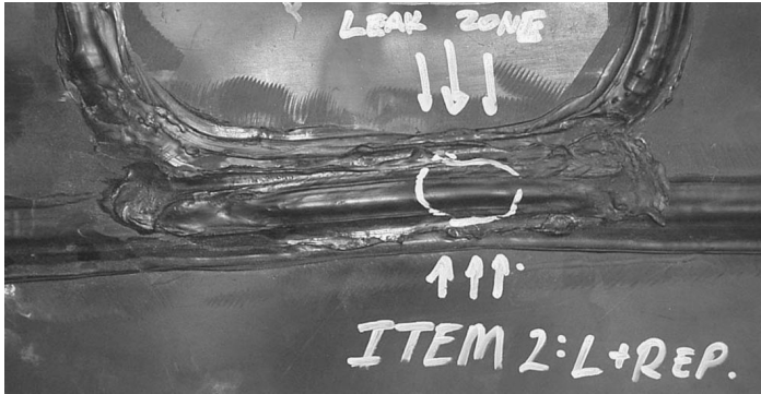
Figure 17.32 Photograph of an example of a poorly made extrusion weld which resulted in a leak zone
