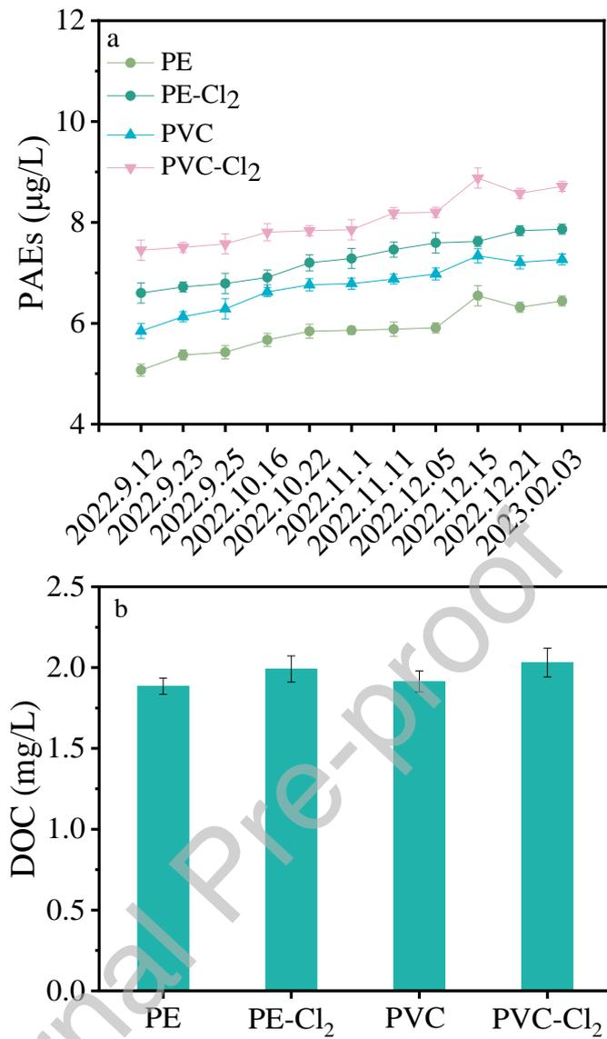
**Fig. 1.** (a) The concentration of total released phthalate acid esters (PAEs), and (b) the dissolved organic carbon (DOC) concentration in effluents of different groups of drinking water distribution pipes after 48 h running.
