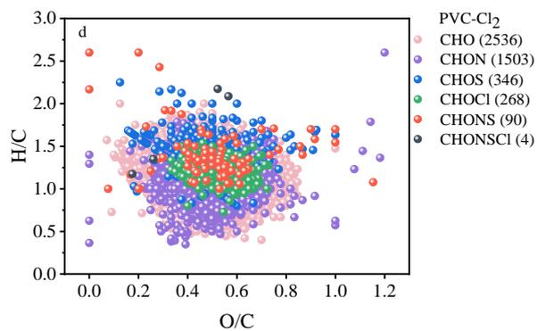
**Fig. 2.** Van Krevelen diagrams of the molecular formulas of dissolved organic matter (DOM) composition in different groups of water samples for (a) PE, (b) PE-Cl<sub>2</sub>, (c) PVC, and (d) PVC- PE-Cl<sub>2</sub> pipes.
