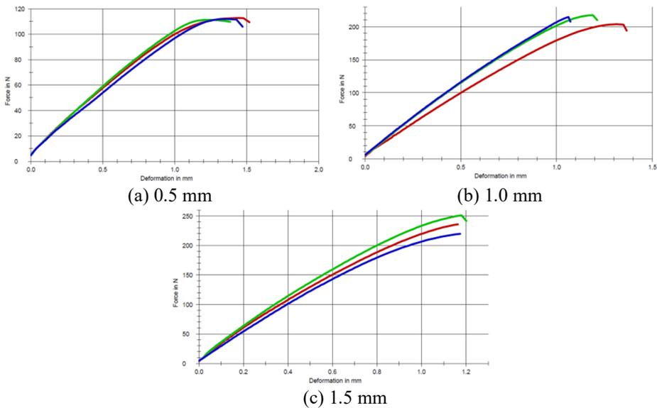
**Fig. 7.** Tensile test force-deformation curve of 3D printed PLA geomembrane.
