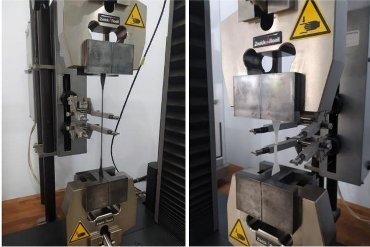
**Fig. 5.** Testing of tensile strength for HDPE and PLA geomembranes.
