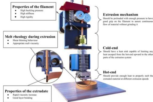
**Fig. 3.** FFF 3D printer [24].
