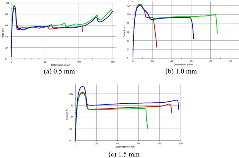
**Fig. 6.** Tensile test force-deformation curve of HDPE geomembrane.
