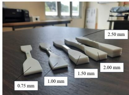
**Fig. 4.** Results of tensile test samples using 3D printing.
