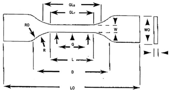
Fig. 2. Geometry of dog bone tensile test sample based on ASTM D 6693-03.
