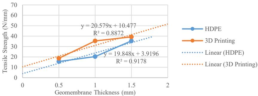
**Fig. 8.** Comparison analysis of HDPE and 3D printed PLA geomembranes.
