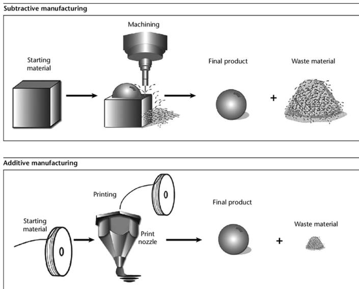
**Fig. 1.** Subtractive and additive manufacturing processes [10].
