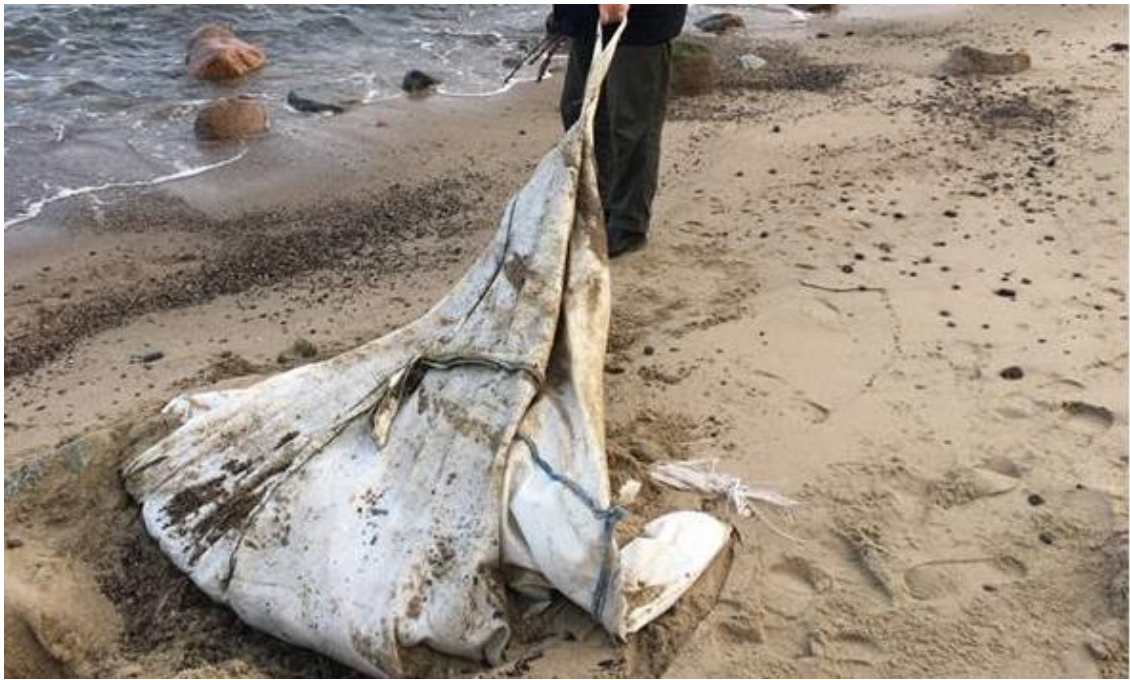
Figure 1.13. Used geotextile (a woven bag, HDPE, PP).
