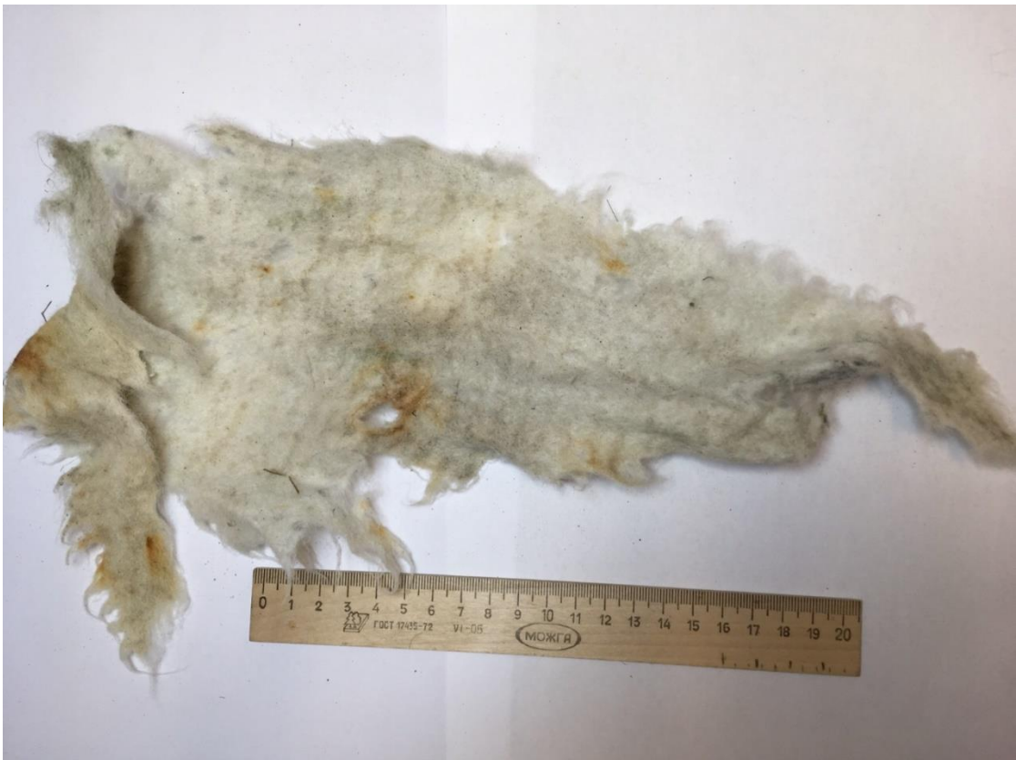
Figure 1.4. The Fragment of black nonwoven geotextile (PP, PET) ). Pieces are not fresh; they were a long time in natural conditions.
