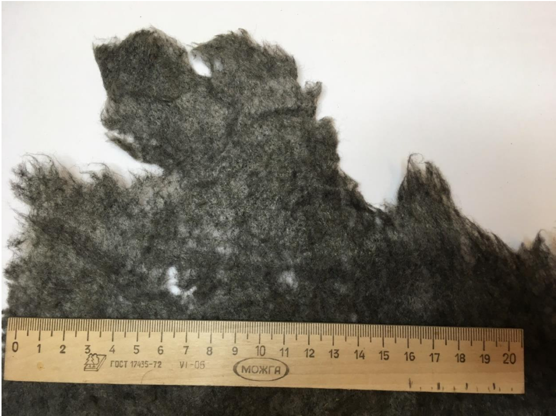
Figure 1.4. The Fragment of black nonwoven geotextile (PP, PET) ). Pieces are not fresh; they were a long time in natural conditions.
