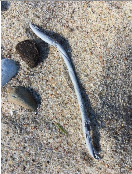
Figure 1.10. Examples of the gabion fragments on the beaches of the Kaliningrad Oblast, Russia.
