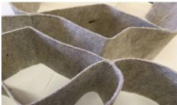
Figure 1.14. Geocells are made from PP, HDPE or PE fibres.
