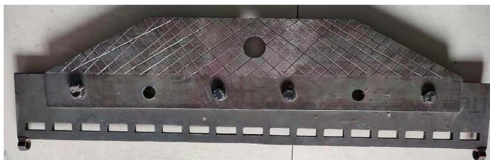
**Figure 3.** The special clamp used for the hexagonal gabion mesh.
