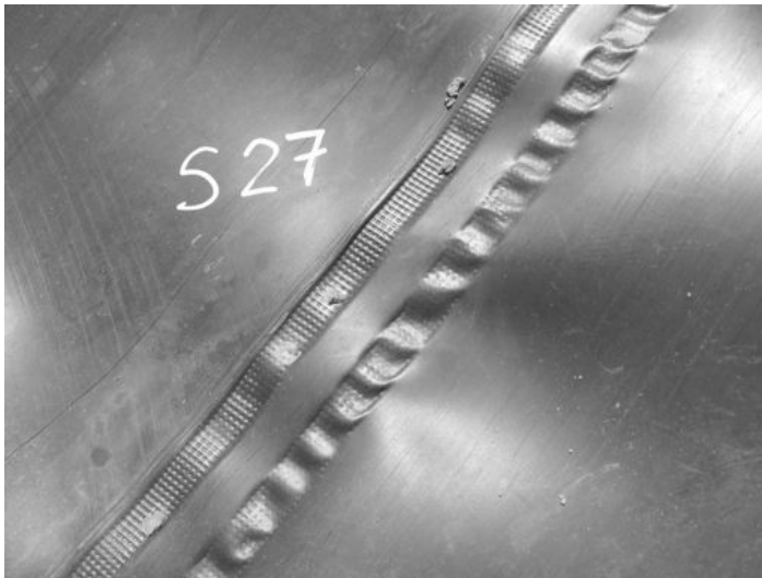
Figure 17.12 Photograph of weld tracks formed by hot wedge welding of 1 mm HDPE geomembranes. Note the poor tracking of the nip roller for the lower weld track
