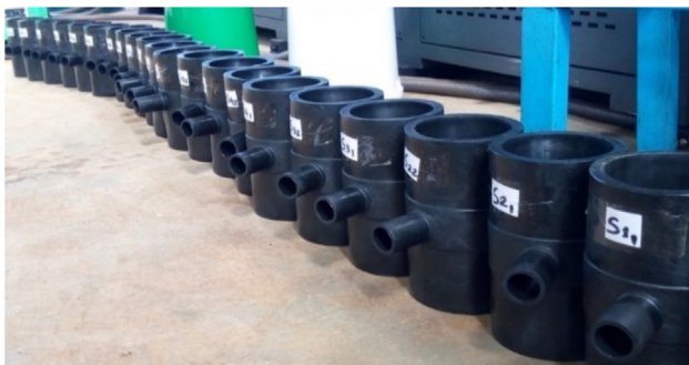
Fig. 6. Produced T-Reducer samples.
