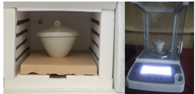
Fig. 4. Ash content test (a) Crucible in the furnace (b) measuring the mass of crucible and materials to be tested.
