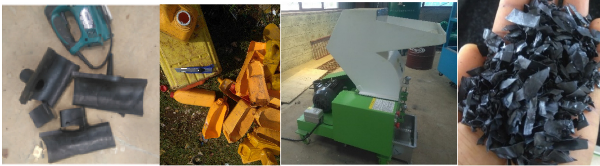
Fig. 2. Suze reduction and Shredding of waste plastic.
