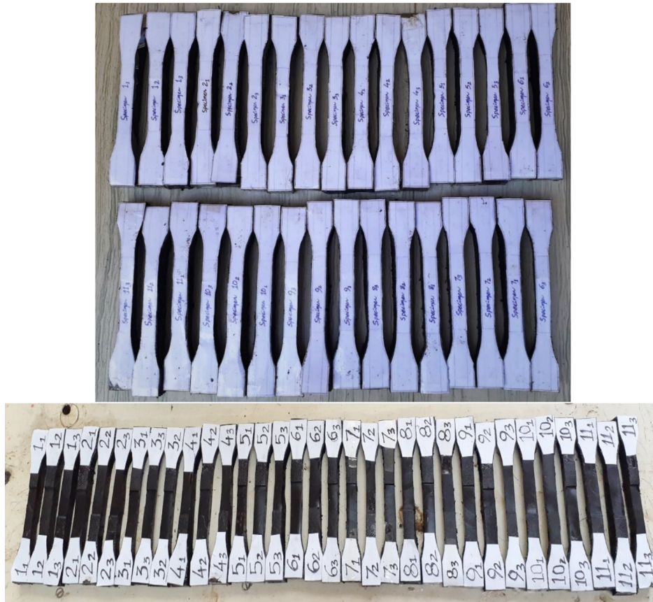
Fig. 8. All tensile test specimens.
