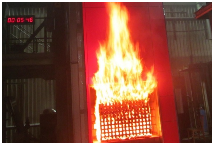
A BS 8414 test underway (picture: BRE)
