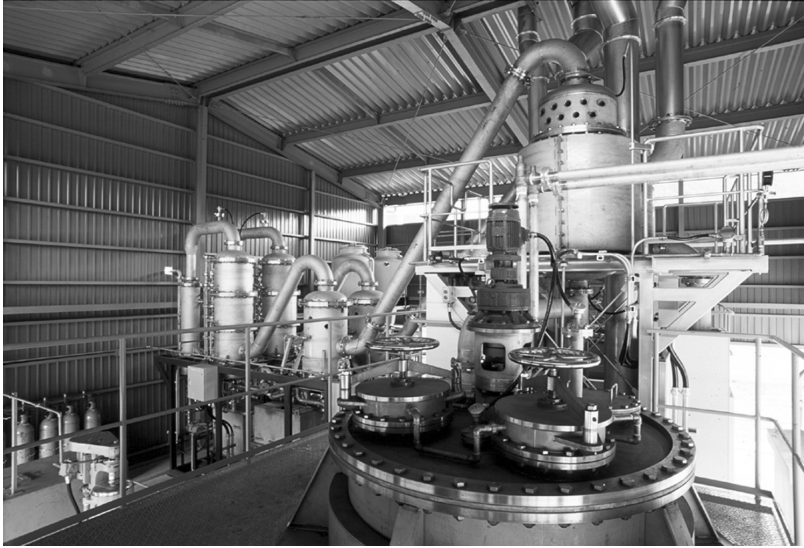
Figure 15.7 Close-up of catalytic reaction tower and condensers of the Thermofuel process. (Reproduced by permission of Ozmotech Pty Ltd)
