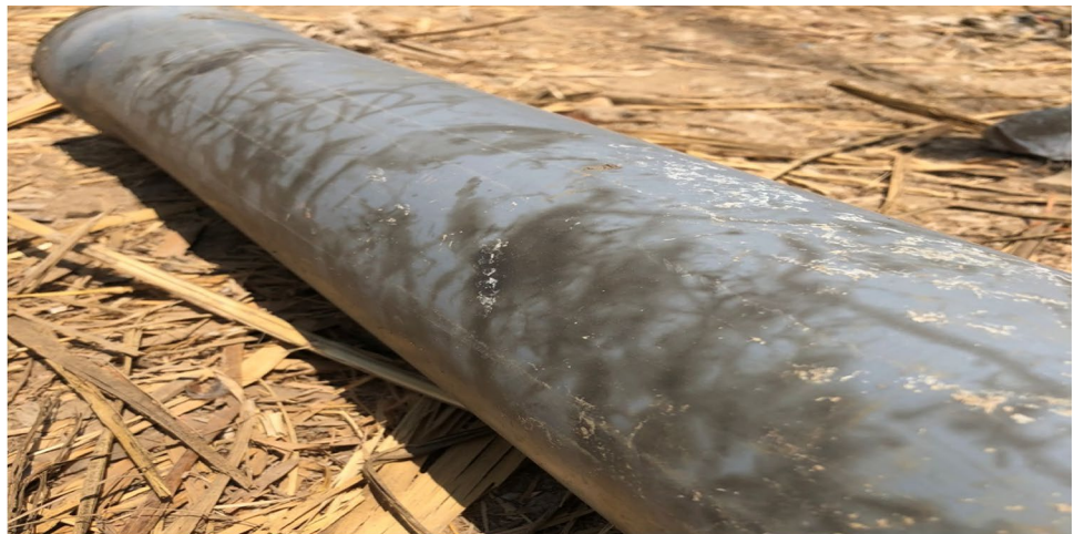
Fig. 11 The dark random streams on the outer surface of the aged uPVC pipes
