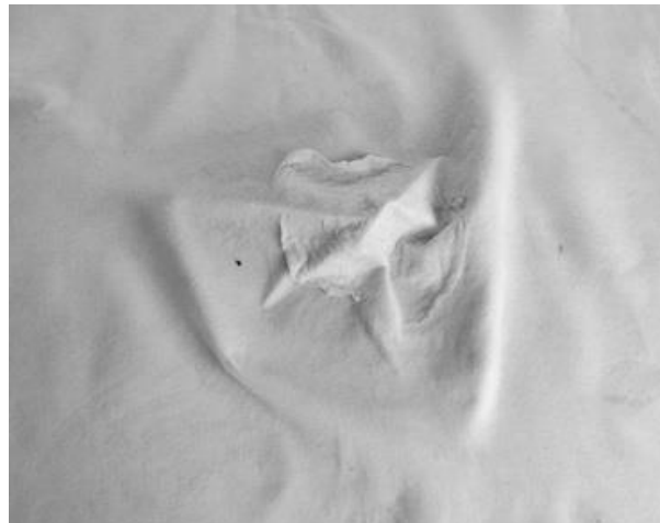
Figure 3. Specimen showing the effects of abrasive shearing on the subgrade side of the geotextile. This specimen had no puncture and appeared relatively undamaged on the opposite side.
