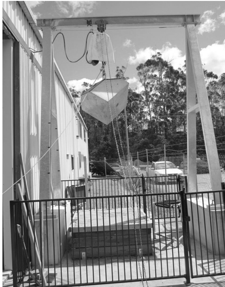
Figure 1. Concrete test cube suspended over the subgrade container with no geotextile in place.
