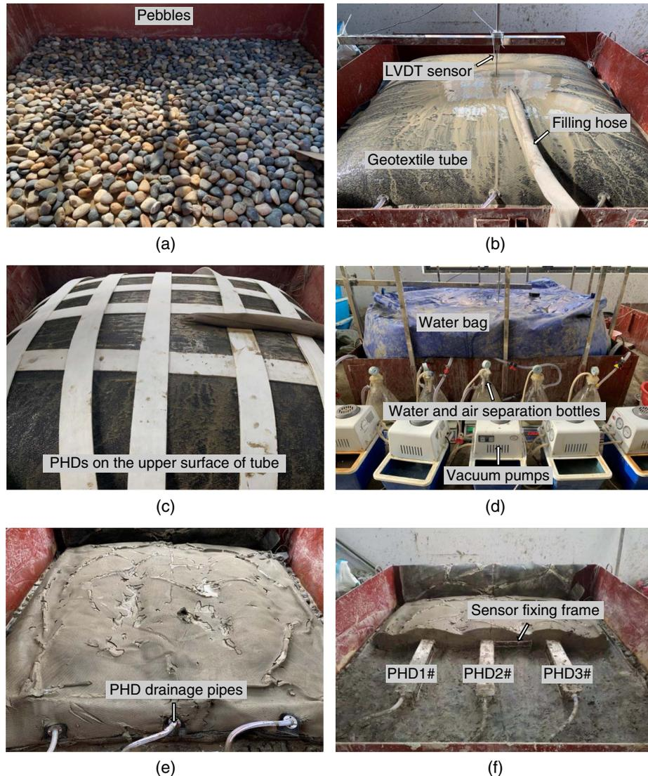
**Fig. 4.** Dewatering implementation process of LT1 for (a) pebbles at the bottom of the container; (b) slurry grouting; (c) PHDs laid on the surface of the geotextile tube; (d) combined vacuum and surcharge preloading; (e) end of the dewatering; and (f) profile of the final state soil.
