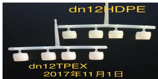
Figure10: The injection molding products of HDPE and TPEX
