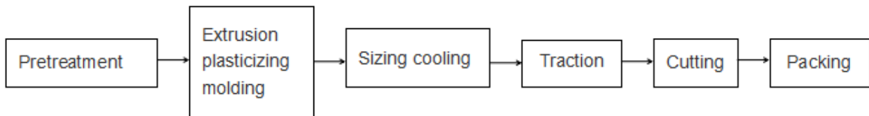
Figure 6: Flow chart of TPEX pipe manufacturing process
