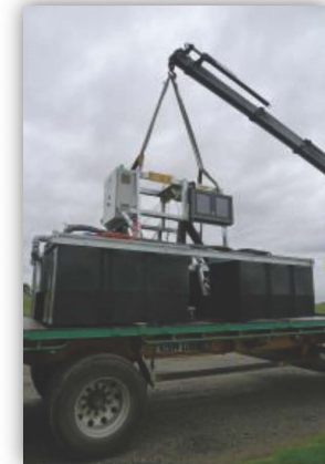
The SlurryCat™ 4000 – Type 1 can be transported to any work site on a standard semi-truck/trailer
