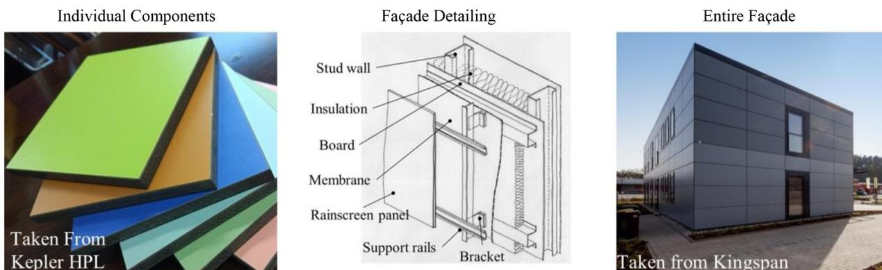
**Figure 2.** Images demonstrating the different levels of analysis when considering a façade. Currently, fire research focuses mainly on individual components, while large scale fire testing is used to assess façade systems.
