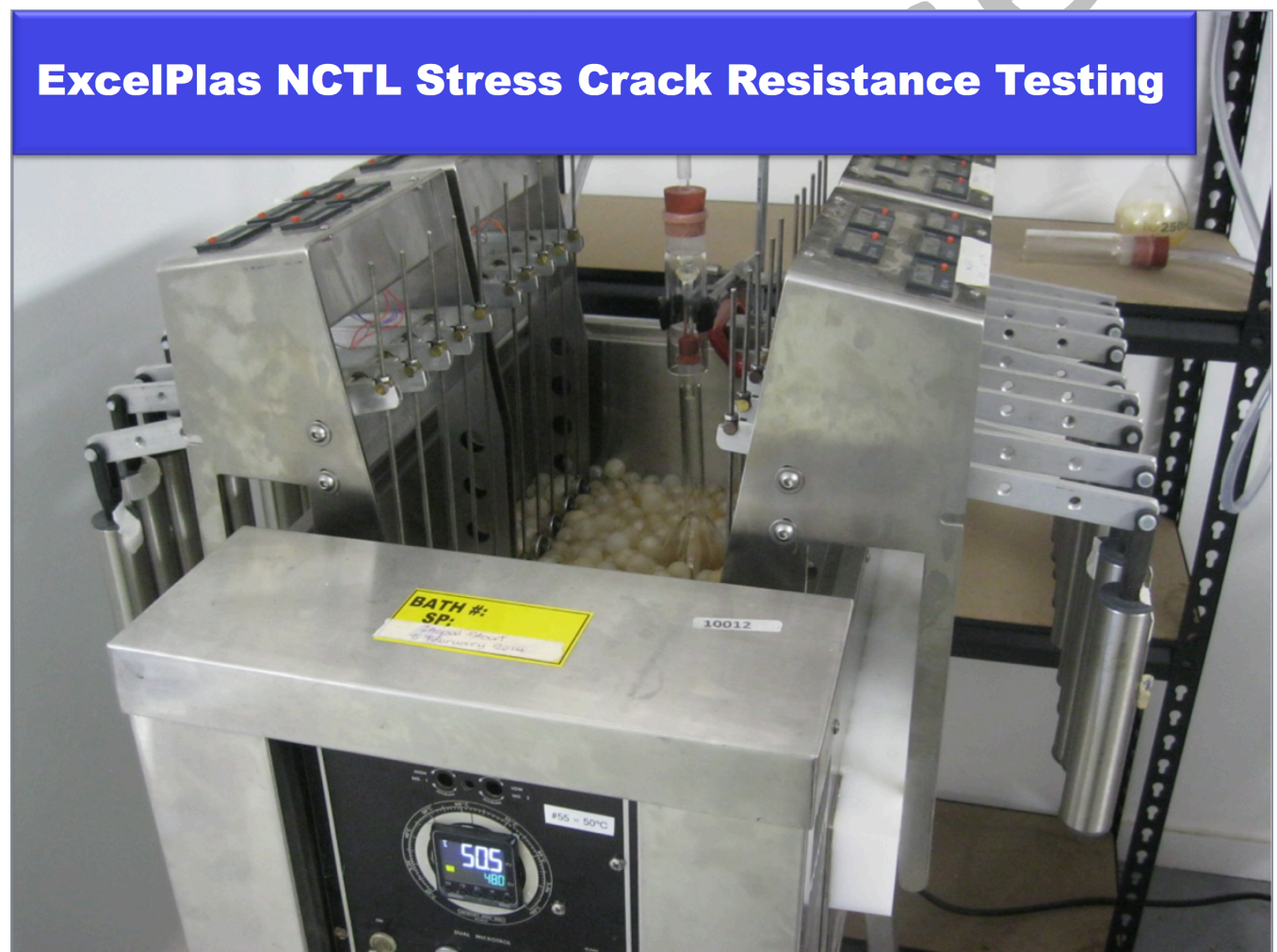
Figure 3. NCTL-SCR specimens under test in 50 deg.C thermostatted Igepal™ bath.
